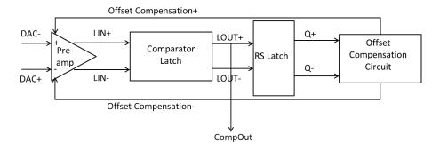
Figure 4.5: Comparator block architecture.
