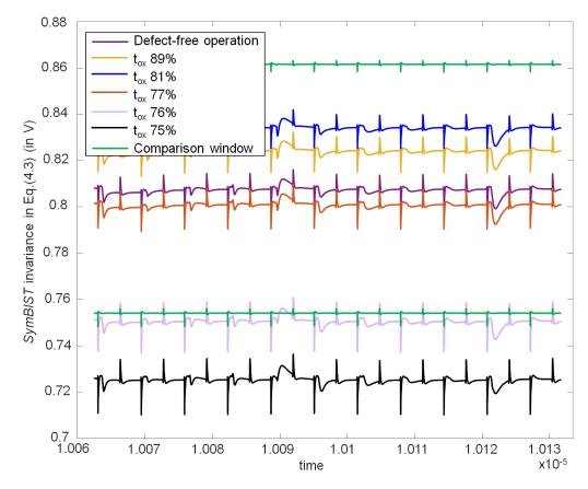
Figure 6.9: SymBIST response to a latent defect.
