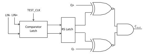
Figure 4.8: Checker design for the invariance in Equation (4.9).
