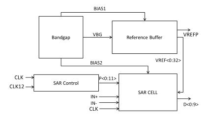
Figure 4.2: Top-level architecture of the SAR ADC IP.
