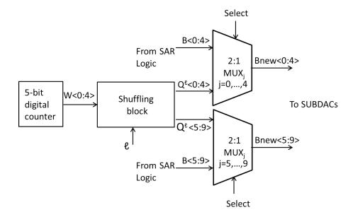
Figure 4.6: On-chip generation of dynamic test stimulus.
