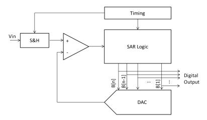
Figure 4.1: High-level architecture of a SAR ADC.
