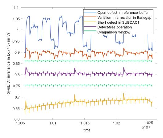
Figure 6.3: Transient simulation of *SymBIST* invariance in Equation (4.3) for different defect scenarios and blocks.
