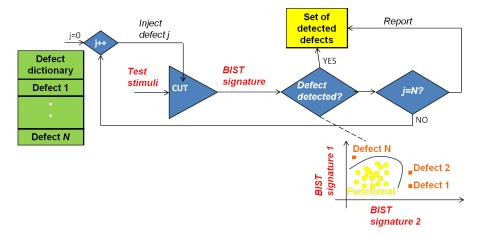
Figure 5.1: Defect Simulation Workflow.
