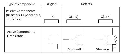
Figure 5.2: Defect model from [7].
