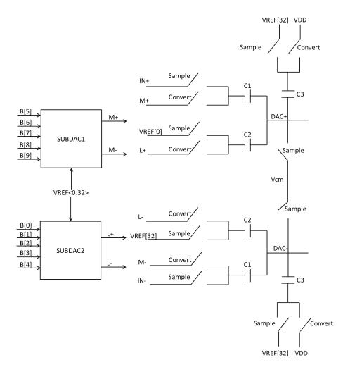
Figure 4.4: 10-bit DAC block architecture.
