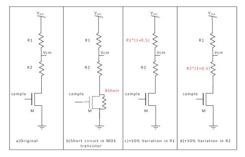
Figure 5.3: Injection of defects 5.1 and 5.2.
