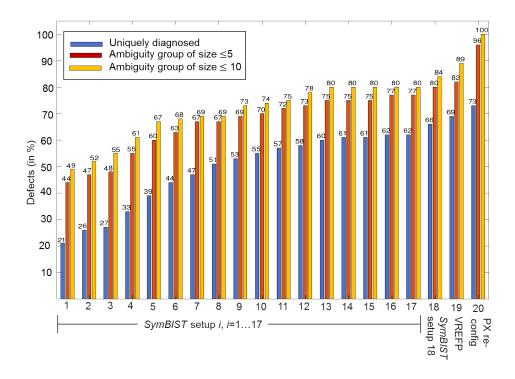
Figure 6.12: Percentage of defects uniquely diagnosed and in ambiguity groups of sizes  $\leq 5$  and  $\leq 10$ .
