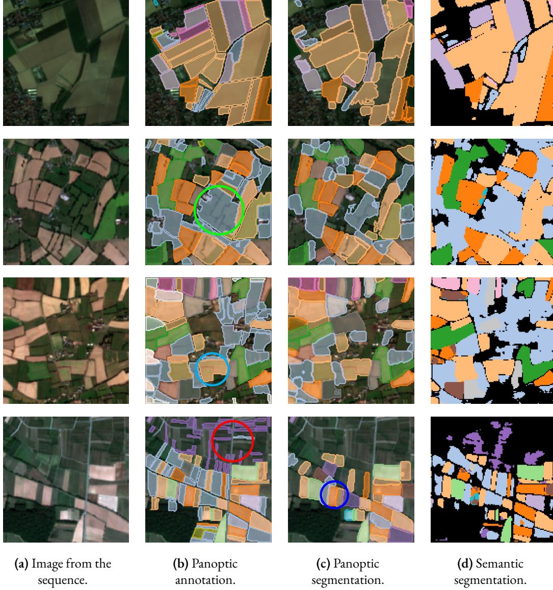
Figure 2.12: Qualitative Panoptic Segmentation Results. We represent a single image from the sequence using the RGB channels (a), and whose ground truth parcel’s limit and types are known (b). We then show the parcels predicted by our panoptic segmentation model (c), and the pixelwise prediction of U-TAE (d). See Figure 2.4 for the color to crop type correspondence. We highlight with a green circle ○ a large, fragmented parcel declared as one single field. This leads to predictions with low confidence and a low panoptic quality. Conversely, the cyan circle ○ highlights such fragmented parcel which is correctly predicted as a single instance. This suggests that our network is able to use the temporal dynamics to recover ambiguous borders. We highlight a failure case with the red circle ○ , for which many thin parcels are not properly detected, resulting in a low panoptic quality. We observe that the semantic segmentation model struggles as well for such thin parcels. Finally, we highlight with a blue circle ○ an example in which the panoptic prediction is superior to the semantic segmentation, indicating that detecting parcels’ boundaries and extent can be informative for their classification.
