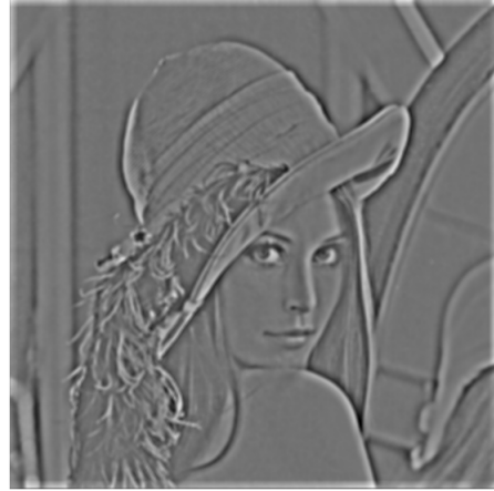
(b) img2 : img1 + filtre Laplacian of Gaussian
