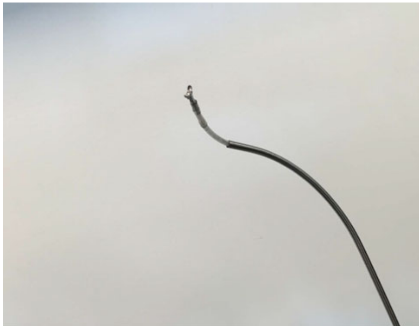
Figure 2.8: A concentric tube robot or Active Cannula composed by 3 pre-curved tubes, from [Wu 2017]
