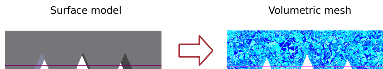
Figure 3.3: Illustration of a mesh. The volumetric mesh is created from a surface model of the manipulator.
