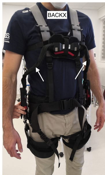
Figure A.3: BackX worn by a participant. The arrows point to the metallic arcs that are constraining the arms during the PP gestures: the participants pointed out that this was one of the main reasons for not choosing to use this exoskeleton for this particular gesture. The BackX was perceived similar to the LAEVO in terms of assistance, but both participants reported that the metallic curved bars from the sternum to the hip were preventing several arm movements necessary to complete the PP maneuver, and as such they felt they could not execute the entire maneuver with this equipment in real conditions.
