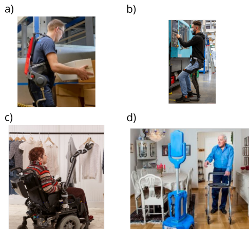
Figure 3: Humans and robots in close proximity in and out of the industrial environment [119]. a) Active exoskeleton that supports lumbar motion at the sagittal plane (German Bionic); b) Active exoskeleton that transforms itself into a stool (Noonee); c) Robotic arm attached to a wheelchair (Kinova); d) Telepresence robot supports independent living for the elder (Giraff Telepresence Robot) .
