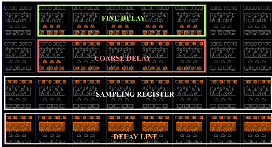
b) FPGA Implemented design of 1 TDC instance
