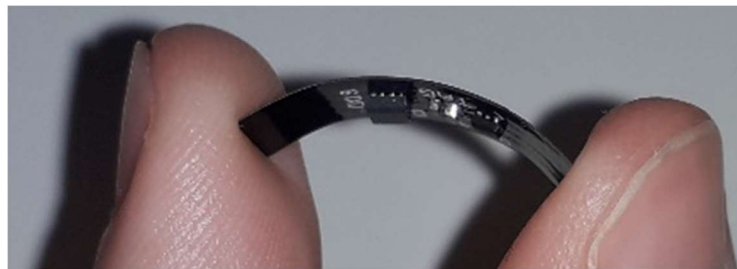
Figure 5-6 Example of a flexible sensor node developed in the AUTONOTEX project for integration into a secure sheet that tracks patient activity.
