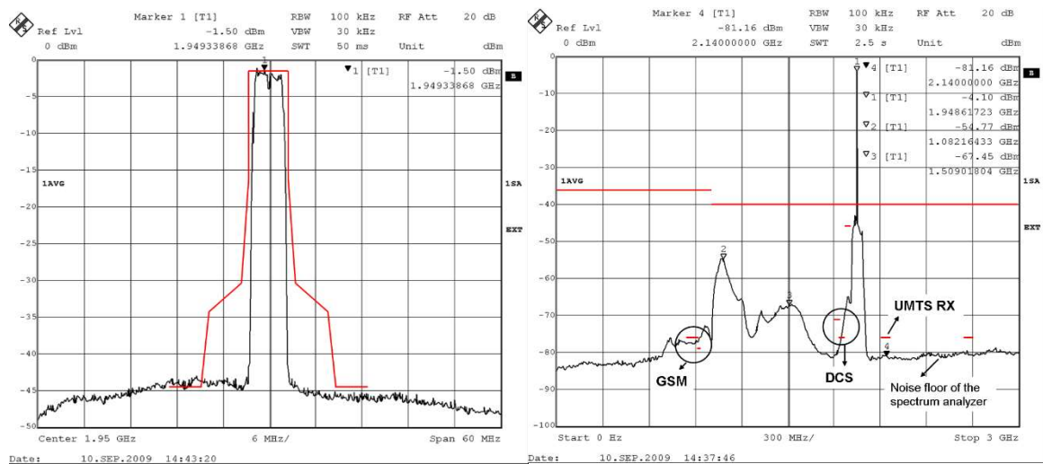
Figure 3-33 Output spectrum of the complete transmitter. (left) Zoom on the bandwidth and (right) full span.
