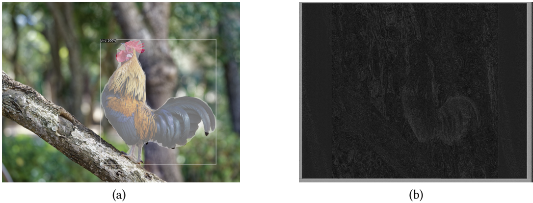
Figure 2.10 – A reference image given to the semantic segmentation and classification framework Mask-RCNN [He+17]. (a) The rooster is detected as "bird" and relatively well segmented. (b) The eavesdropped counterpart of the reference image. Nothing is detected by the Mask-RCNN instance.
