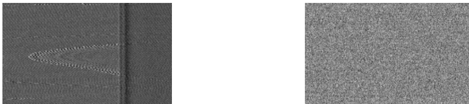
Figure 2.9 – Examples of corruptions contained in an eavesdropped image. Left: unknown interference noise, right: hybrid Gaussian (thermal) and Bernoulli (saturation) noise.
