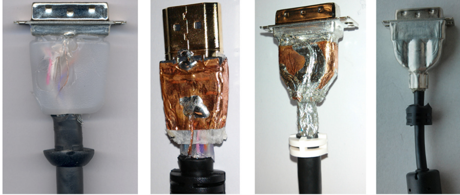
Figure 2.3 – Different video connectors that may lead to compromising emanations. Images from Pierre-Michel Ricordel and Emmanuel Duponchelle [RD18].
