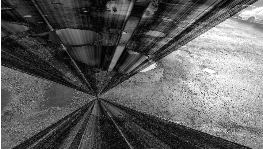
FIGURE 4.5: Inaccurate alignment through homography estimation.
