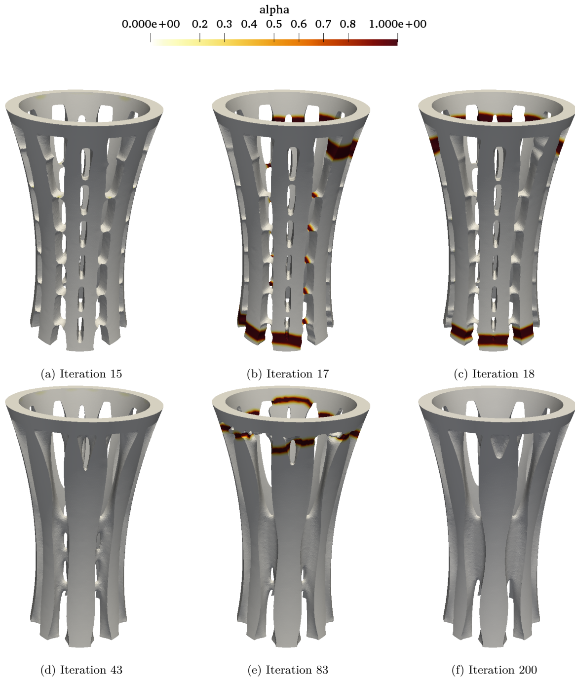
Figure 7.11: Damage parameter \alpha at the last time instant plotted for several optimization iterations for the shape in Fig.7.10b
