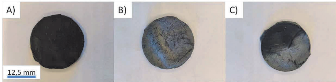
Figure 36: PE(A)-CNT (0.6 vol % CNT) samples with 1 vol % SA (A); 5 vol % SA (B). Picture C) is the sample B) half wiped.
