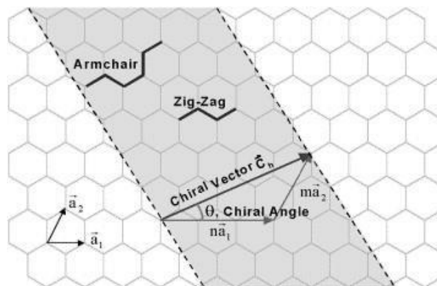
Figure 4: Schematic diagram showing how a hexagonal sheet of graphite is 'rolled' to form a carbon nanotube [7]
