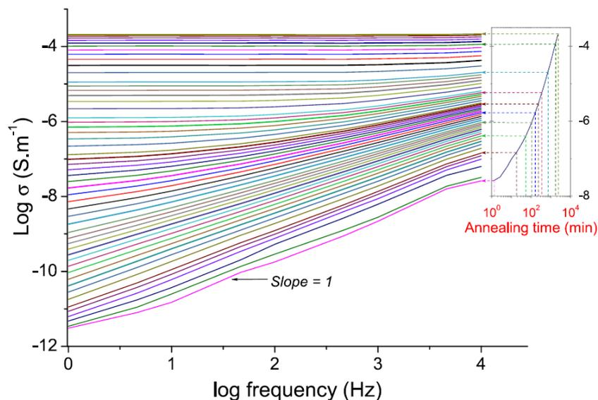
Figure 14: Change in frequency dependence of the conductivity of a composite sample filled with a steady content of 2.2wt. % of MWCNT and annealed at  $150^\circ\text{C}$  (inset is conductivity as a function of time for  $f=10^4 \text{ Hz}$ ). reproduced from [96].
