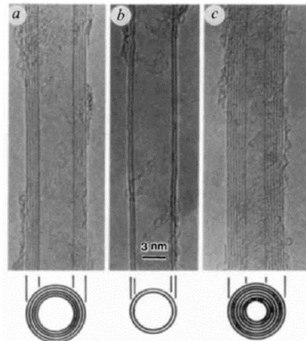
*Figure 3: First TEM picture of carbon nanotubes. Cross section of nanotubes with dark lines representing the (002) lattice images of graphite. a), b) and c) are Carbon nanotubes containing respectively 5, 2 and 7 graphitic sheets [1]*
