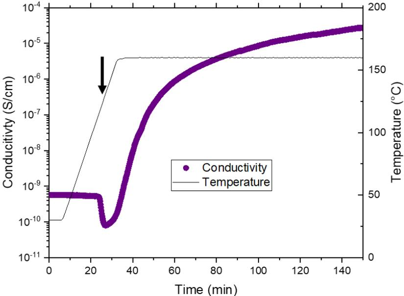
Figure 32: Conductivity change during annealing treatment (2 hours - 160°C) for PE (C) -CNT (0.15 vol % CNT).  $f = 1$  kHz. The black arrow outlines the time when the temperature reaches the melting temperature of the PE.
