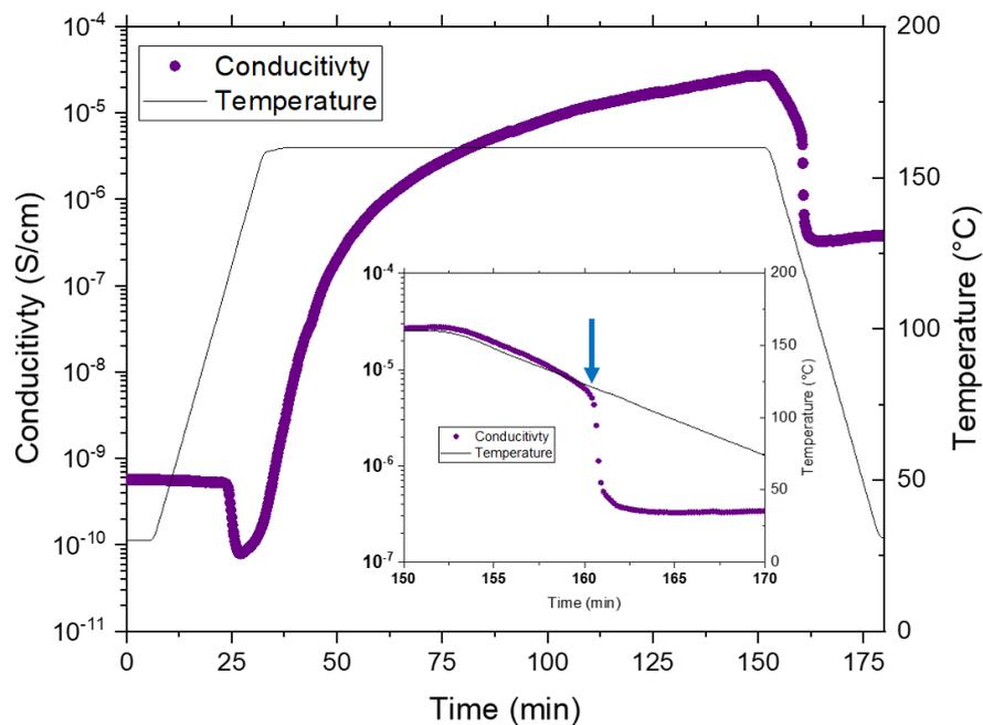
Figure 42: Conductivity ( $f= 1$  kHz) evolution during an annealing treatment (at  $160^{\circ}\text{C}$  for 120 minutes) and the following cooling down to room temperature for LLDPE(C)-CNT (0,15 vol %). As inset is plotted a zoom of the cooling step. The blue arrow outlines the crystallization temperature.
