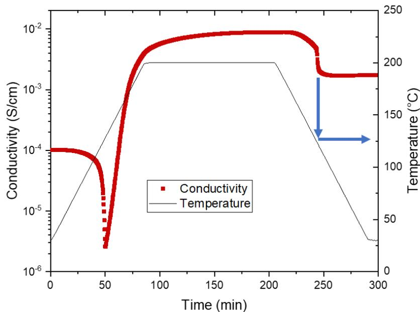
Figure 39: Conductivity evolution during annealing treatment (200°C) and the following cooling down to 30 °C for PE(A)-CNT (1.45 vol % CNT).  $f = 1$  kHz. Blue arrows outline the polymer crystallization.
