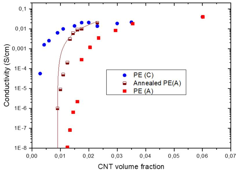
Figure 30: Impact of the annealing for two hours on the conductivity of PE-CNT composites as function of the CNT content. Red line is the percolation law obtained from the fitting of experimental data.
