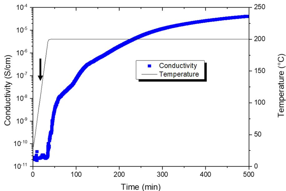
Figure 28: Conductivity change with annealing time at  $200^{\circ}\text{C}$  for PE (A) -CNT ( $0.9$  vol % CNT).  $f= 1$  kHz. The black arrow outlines the time when the temperature reaches the melting temperature of the PE.
