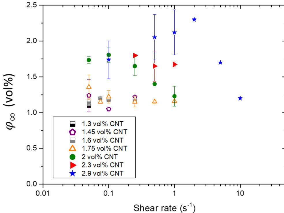
Figure 55: Equilibrium effective fraction versus shear rate for HDPE-CNT composites at various CNT content. The  $\varphi_{\infty}$  parameter was adjusted from **Equation 17** with fixed break up and building parameters. Error bars are standard deviation obtained for repeated experiments.
