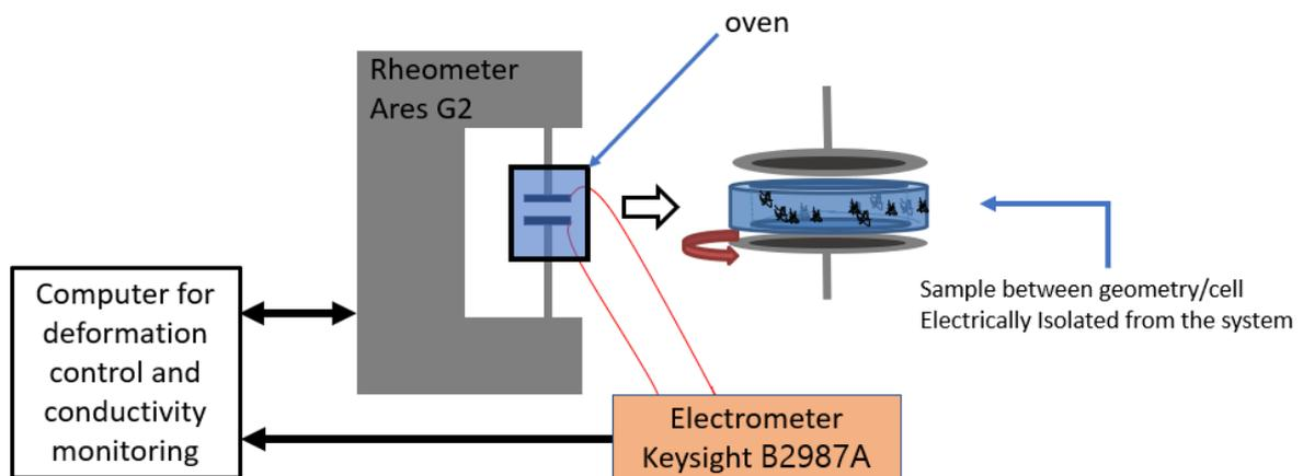
Figure 22: schema of the experimental rheoelectric set-up.
