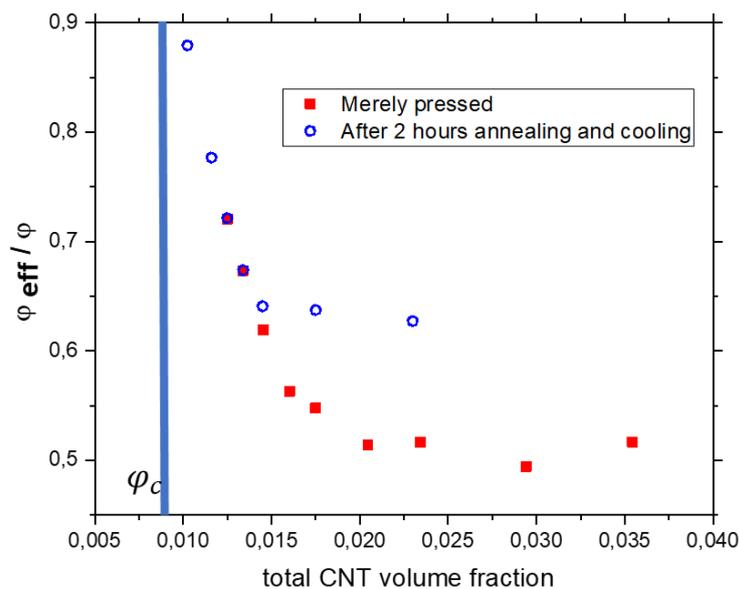
Figure 48: ratio of effective filler fraction over the total CNT content before and after 2 hours annealing treatment (200°C). Effective filler fraction is calculated using the percolation law determined from 2 hours annealing XRT 70 data.
