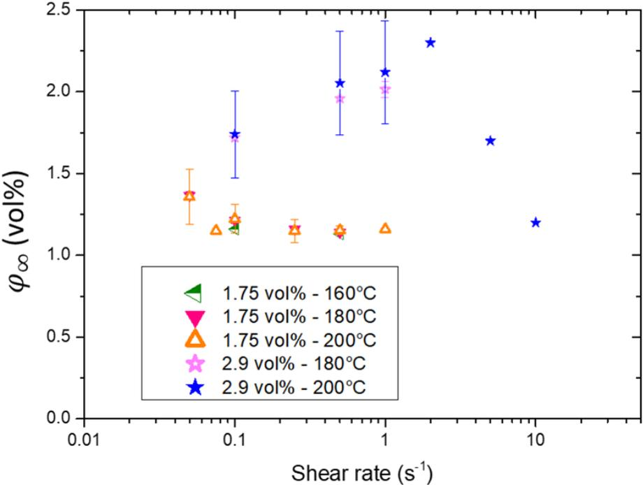
Figure 56: Equilibrium effective fraction versus applied shear rate for experiments at different temperatures. Error bars are standard deviation obtained for repeated experiments.
