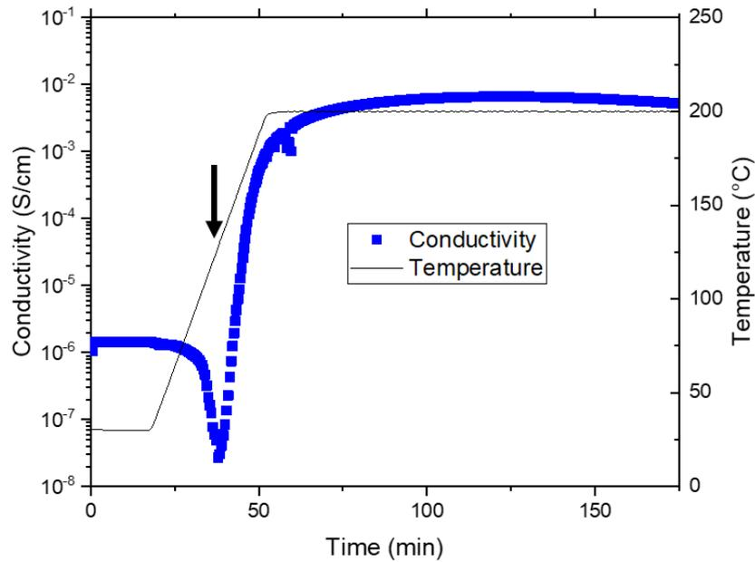
Figure 29: Conductivity change during annealing treatment (2 hours - 200°C) for PE (A) -CNT (1.6 vol % CNT).  $f = 1$  kHz. The black arrow outlines the time when the temperature reaches the melting temperature of the PE.
