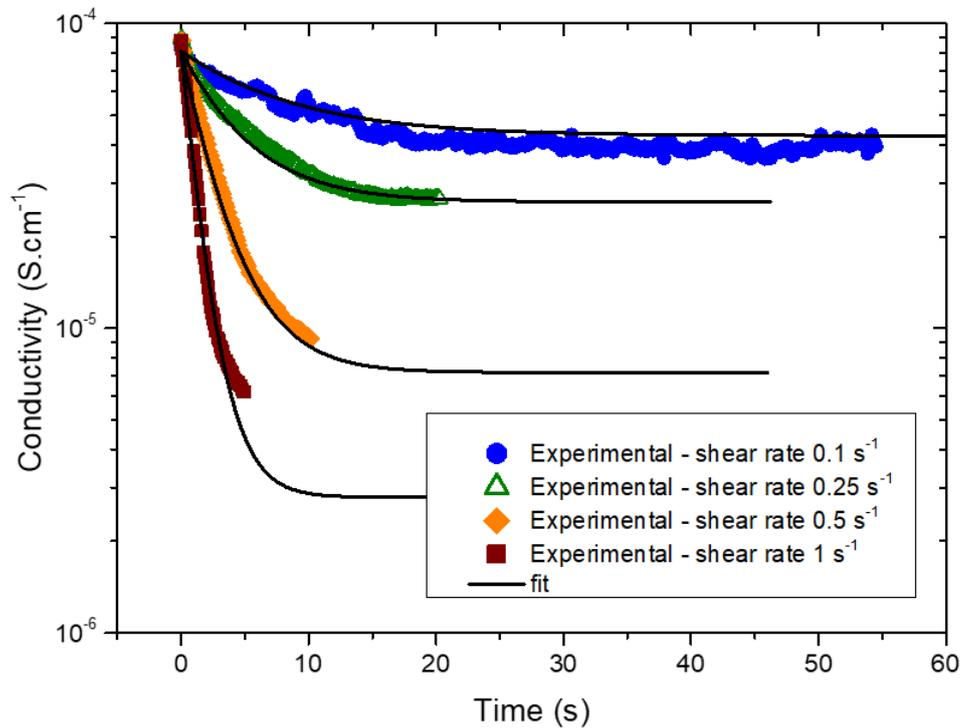
Figure 52: Conductivity variation during shear at 200°C as a function of time for HDPE/CNT (2.0 vol%) at various shear rates for a total strain of 5. Symbols: experimental data; lines: calculated curves with **Equation 17** and parameters shown in **Table 5**
