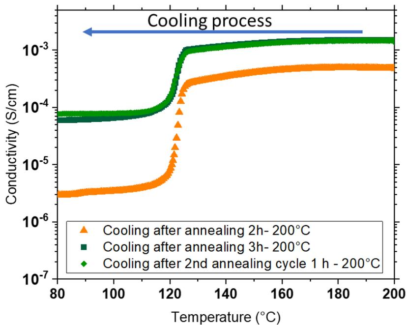
Figure 45: conductivity evolution as function of the temperature during the cooling process from 200°C to 30 °C of PE(A)-CNT composites (1.3 vol% CNT) following different annealing treatments (see Figure 8).
