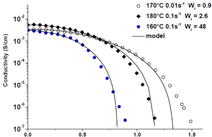
Figure 17: Conductivity variation as a function of the Hencky deformation of PS/MWCNT (0.79 vol%) for large  $W_i$ . Symbols are the experimental data, and the solid lines are the calculated curves. replotted from [111]
