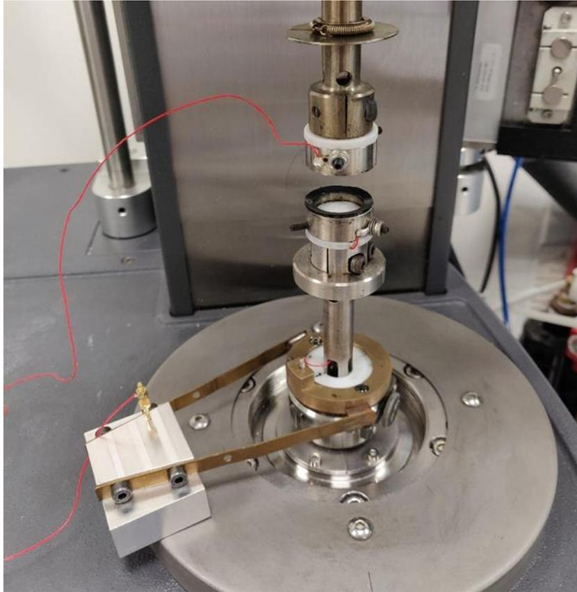
*Figure 23: picture of the rheological cell used for simultaneous conductivity measurement*
