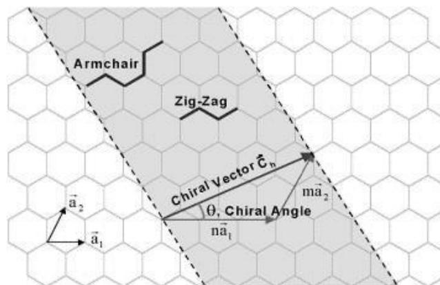
Figure 4: Schematic diagram showing how a hexagonal sheet of graphite is 'rolled' to form a carbon nanotube [7]
