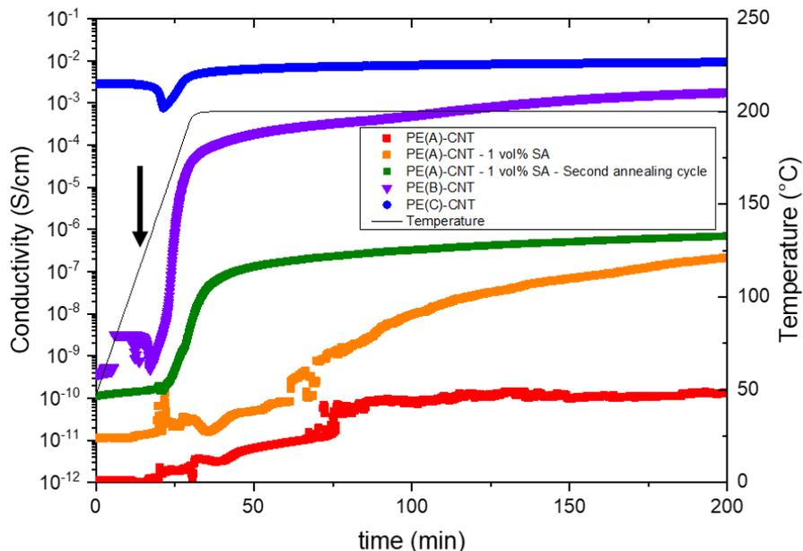
Figure 33: Conductivity evolution during annealing treatment for various PE-CNT (0.6 vol % CNT) systems. The black arrow outlines the time when the temperature reaches the melting temperature of the PE.
