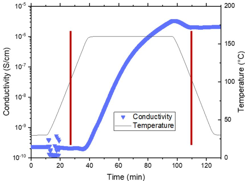
Figure 41: Conductivity ( $f= 1000\text{Hz}$ ) evolution during annealing treatment (at  $160^\circ\text{C}$  for 60 minutes) and cooling down to room temperature for PS-CNT (0,7 vol %). red lines outline the transition above and below the glass transition of the PS.
