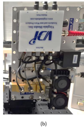
Figure III.2.5 (a) A plot of the VDI AMC source THz output power as a function of its emission frequency. (b) Photograph of the VDI AMC source
