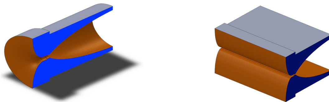
Figure 3.5 – An example of two geometries, on the left an axisymmetric profiled Laval nozzle and on the right a planar profiled nozzle. Both require a convergent part and a divergent calculated profile to generate a uniform supersonic beam expansion.
