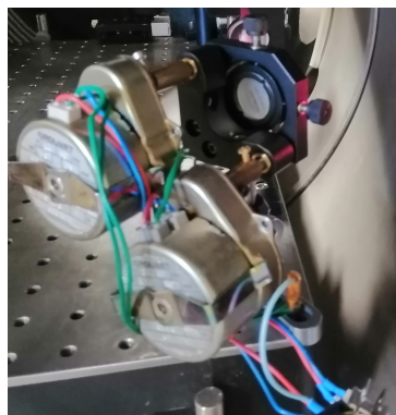
Figure 3.32 – Photo of the two motors fixed on the mirror, making it easy to control and steer the mirror in the x and y direction with a simple controller outside of the chamber
