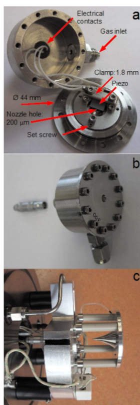
Figure 2.5 – a) Photo of the inside of the cantilever piezovalve, with the relevant dimensions indicated. The O-ring is glued to the back side of the piezo, which forms the vacuum seal to the nozzle hole. The nozzle to seal distance can be carefully adjusted with three set screws as indicated. The piezo free cantilever length is about 5 to 6 mm. The length of the cantilever can be easily adjusted by moving the clamp. b) Photo of the closed valve which has an outer body diameter of 44 mm. c) Photo of the piezo valve body mounted in a heatable holder on a standard ISO160 vacuum flange. An electrically isolated skimmer is also attached to the holder
