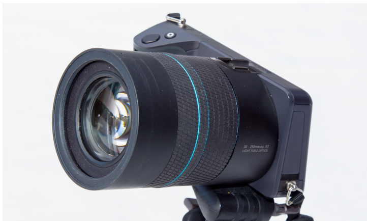
Figure 3 – The Lytro Illum plenoptic camera (source: Wikipedia )
