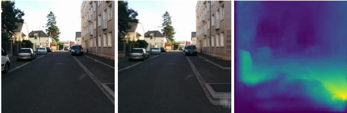
Figure 3.19 – Another example of view synthesis result using our network on natural images captured using a smartphone. From left to right: input image, prediction, depth estimation. We can note that the depth estimation is inaccurate in the foreground, notably in surfaces of the same texture. This error in the depth estimation process has nevertheless few consequences on the finally synthesized image.
