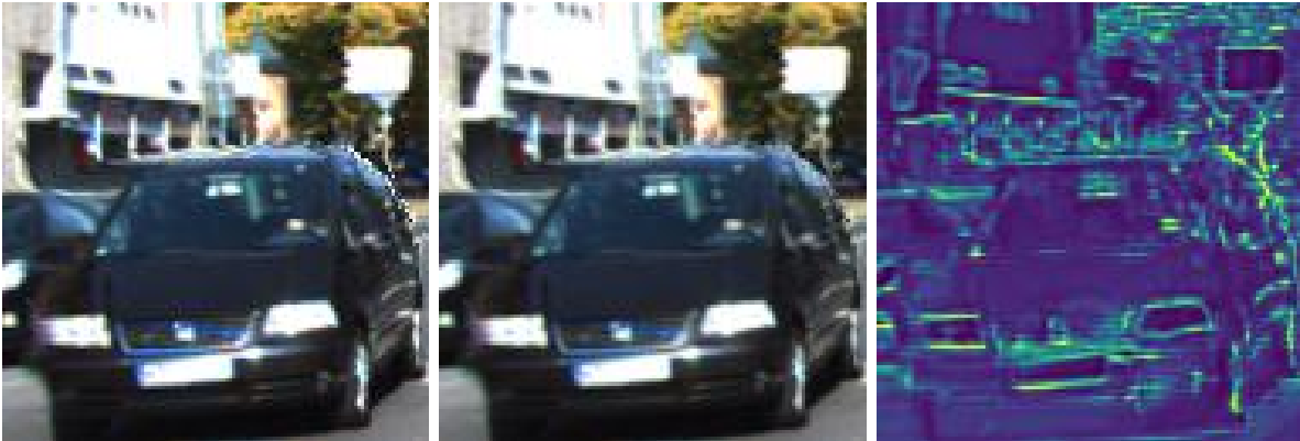
Figure 3.10 – Detail from views to illustrate the contribution of the Refiner. From left to right: prediction from DBP, final prediction, inverted confidence map.
