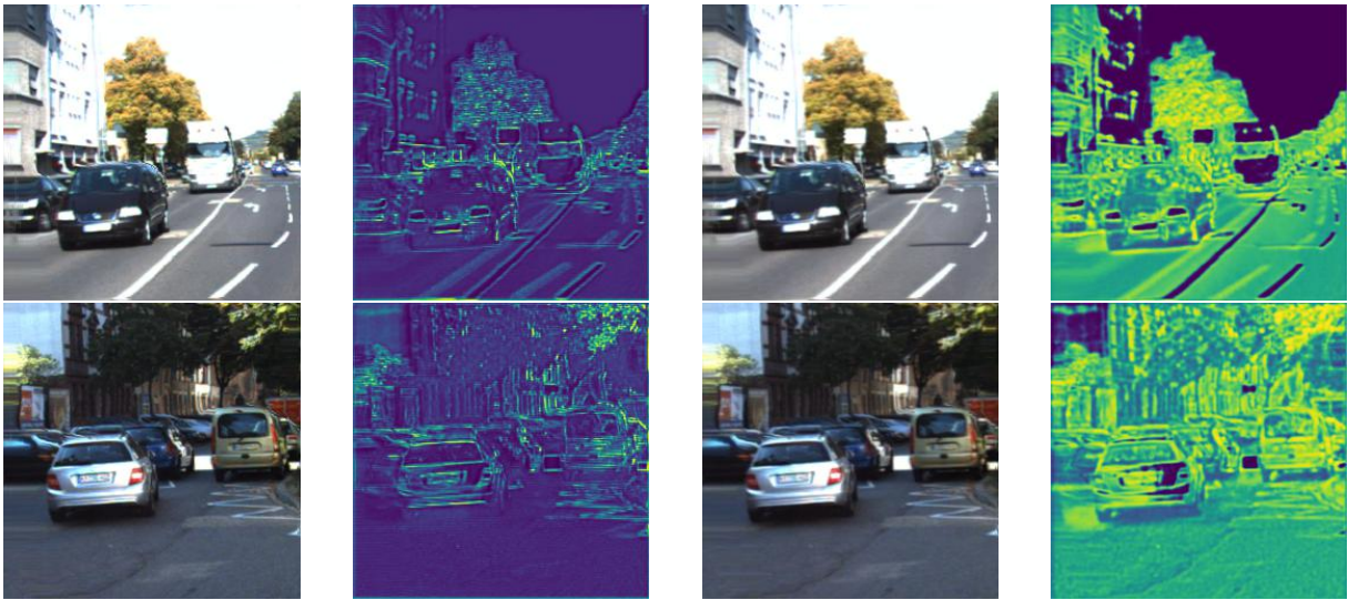
Figure 3.12 – Elements of comparison for constraint set on the confidence map (yellow in confidence maps means low-confidence in DBP prediction). (from left to right: a ) Prediction when FB-constraint is set. b ) Corresponding confidence map. c ) Prediction when no FB-constraint is set. d ) Corresponding confidence map.)
