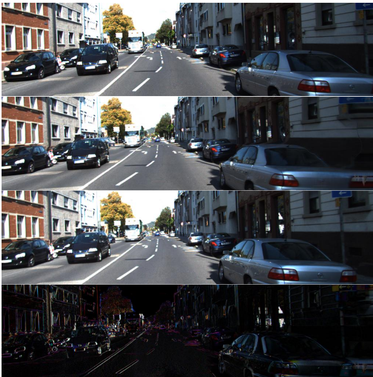
Figure 4.8 – Result of our approach in a stereo setting, on the KITTI test set, for evaluation. From top to bottom: input image, our prediction, ground truth image, L1 error.
