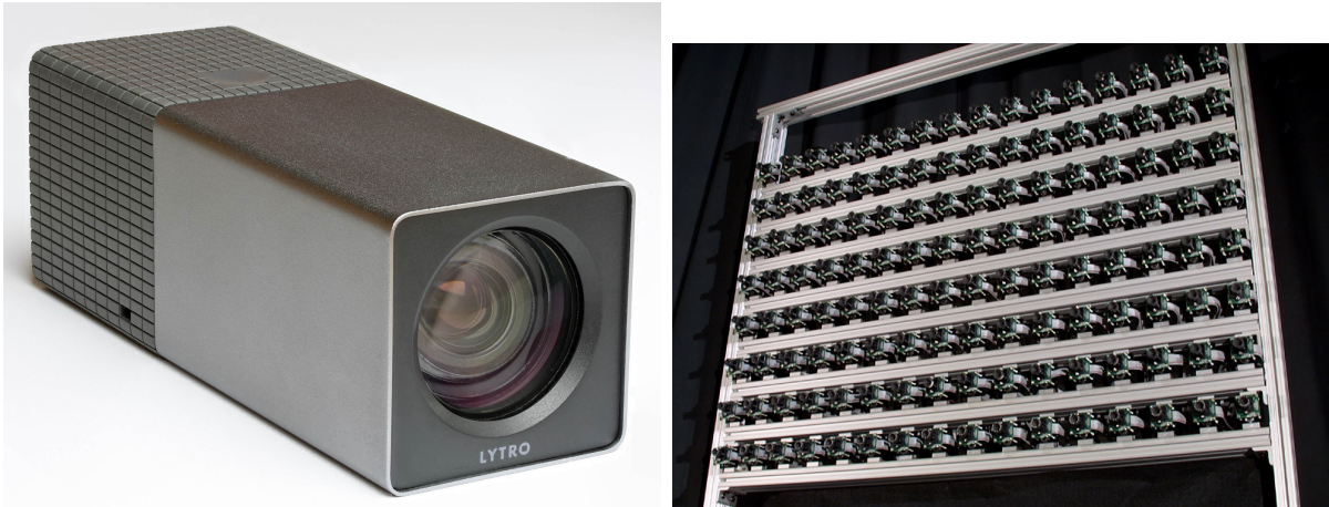
Figure 1.4 – Plenoptic devices: on the left, a Lytro plenoptic camera; on the right, the Stanford camera array, presented in [3].
