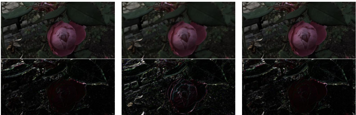
Figure 4.4 – Visual prediction for a top-left image from the Flowers test set, as well as the corresponding L1 errors, for, from left to right, our method, LF4D ([90]) and the stereo version of our method. The errors were multiplied with a factor of 3 for better visualization.
