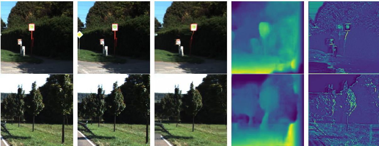
Figure 3.18 – Failure cases for our approach. From left to right: Input image, ground truth image, network prediction, estimated disparity map, confidence map.
