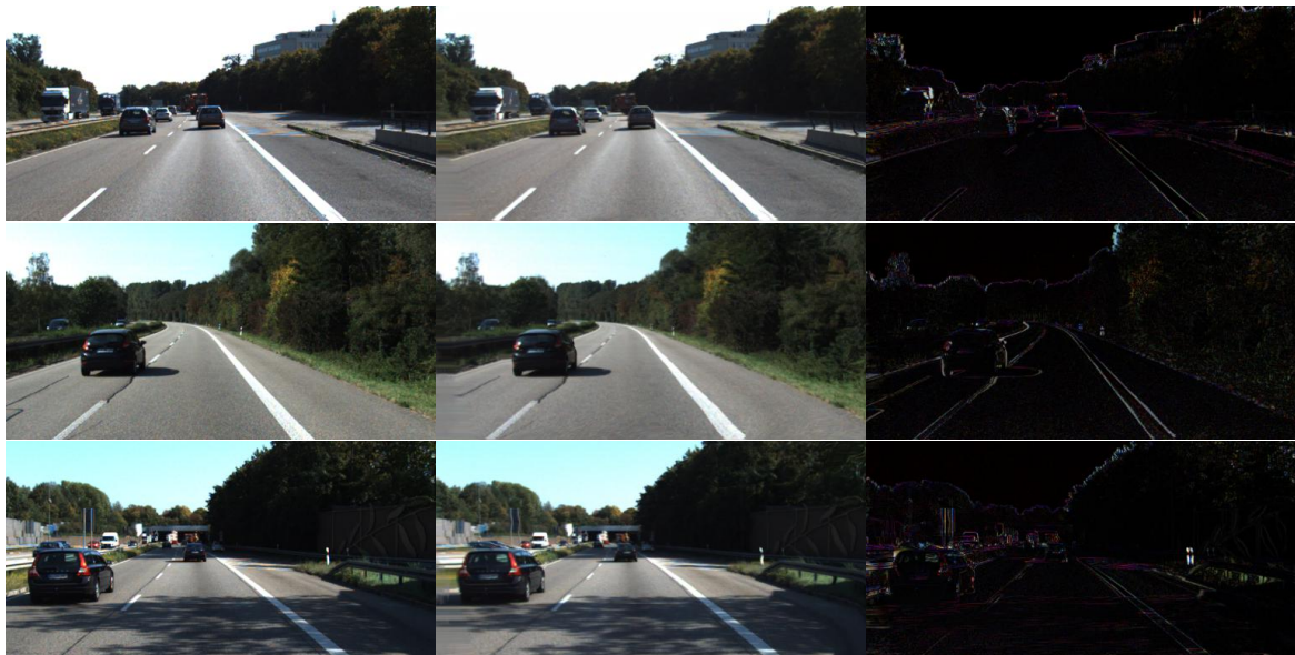
Figure 3.7 – Qualitative evaluation of the predictions carried out. From left to right: ground truth image, our prediction, L1 error between the prediction and the ground truth image.
