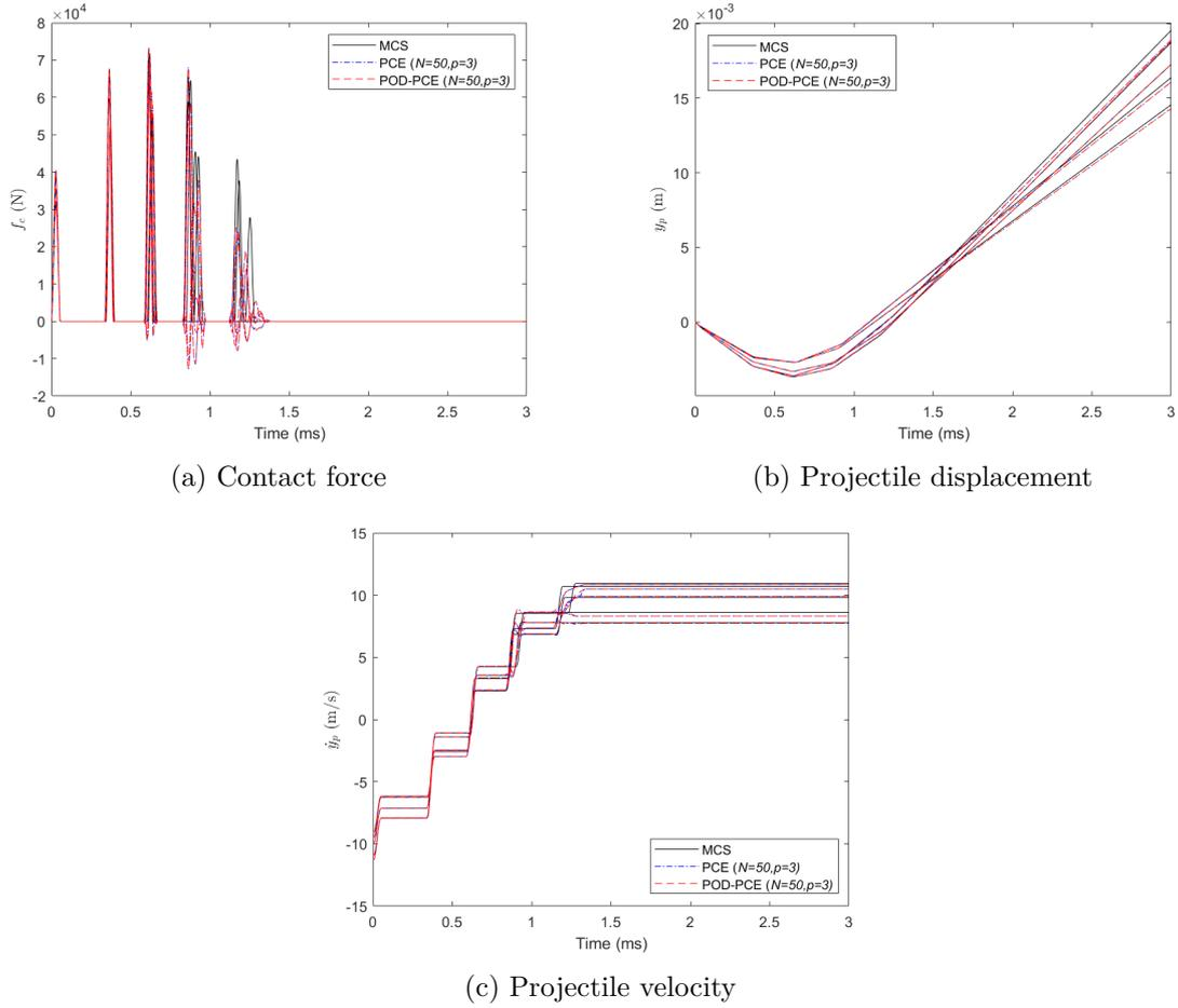
Figure 4.8: Comparison of responses for the multiple impact oscillator at 5 samples:  $m_p \in \{342.71, 292.84, 365.62, 310.35, 373.82\}g$ ,  $k_c \in \{13.97, 13.87, 14.61, 14.23, 13.63\} \times 10^3 \text{MN m}^{-3/2}$ ,  $v_0 \in -\{11.32, 9.51, 9.96, 9.11, 10.95\} \text{m s}^{-1}$
