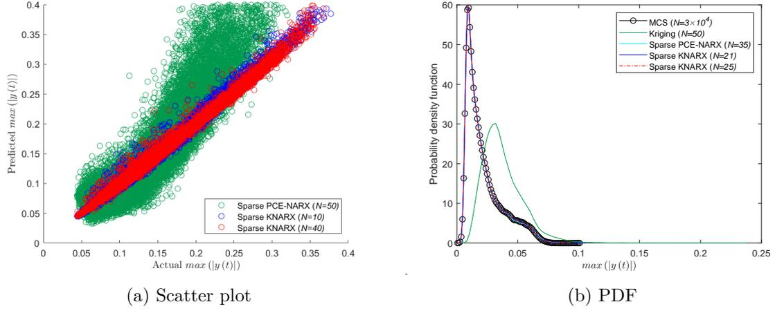
Figure 3.10: Comparison of predicted  $\max(|y(t)|)$  for the Bouc-Wen oscillator
