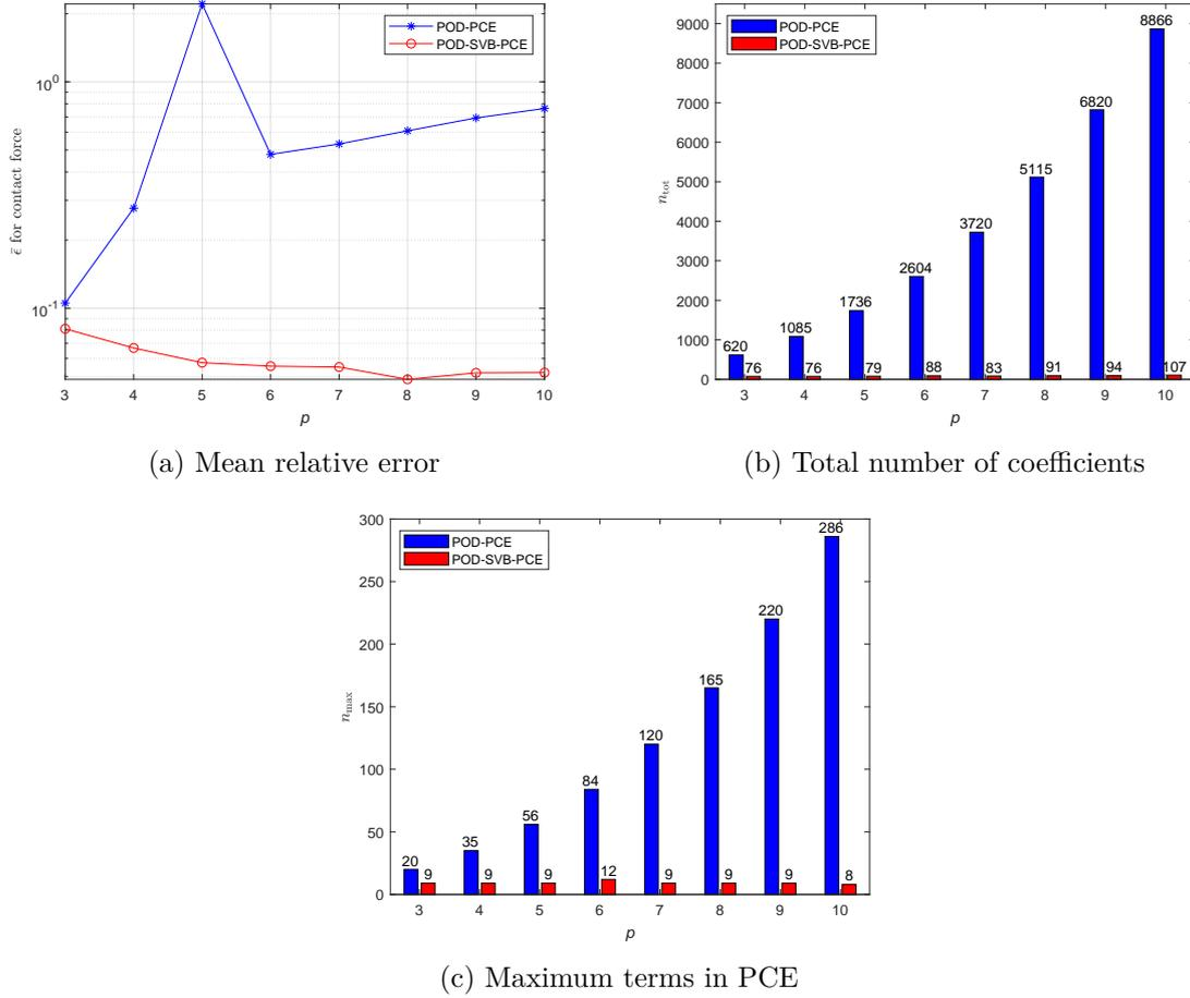
Figure 5.10: Evolution of the mean relative error and the PCE coefficients with the increase of polynomial degree  $p$  for the predicted contact force by the POD-PCE and the POD-SVB-PCE models with  $N = 50$
