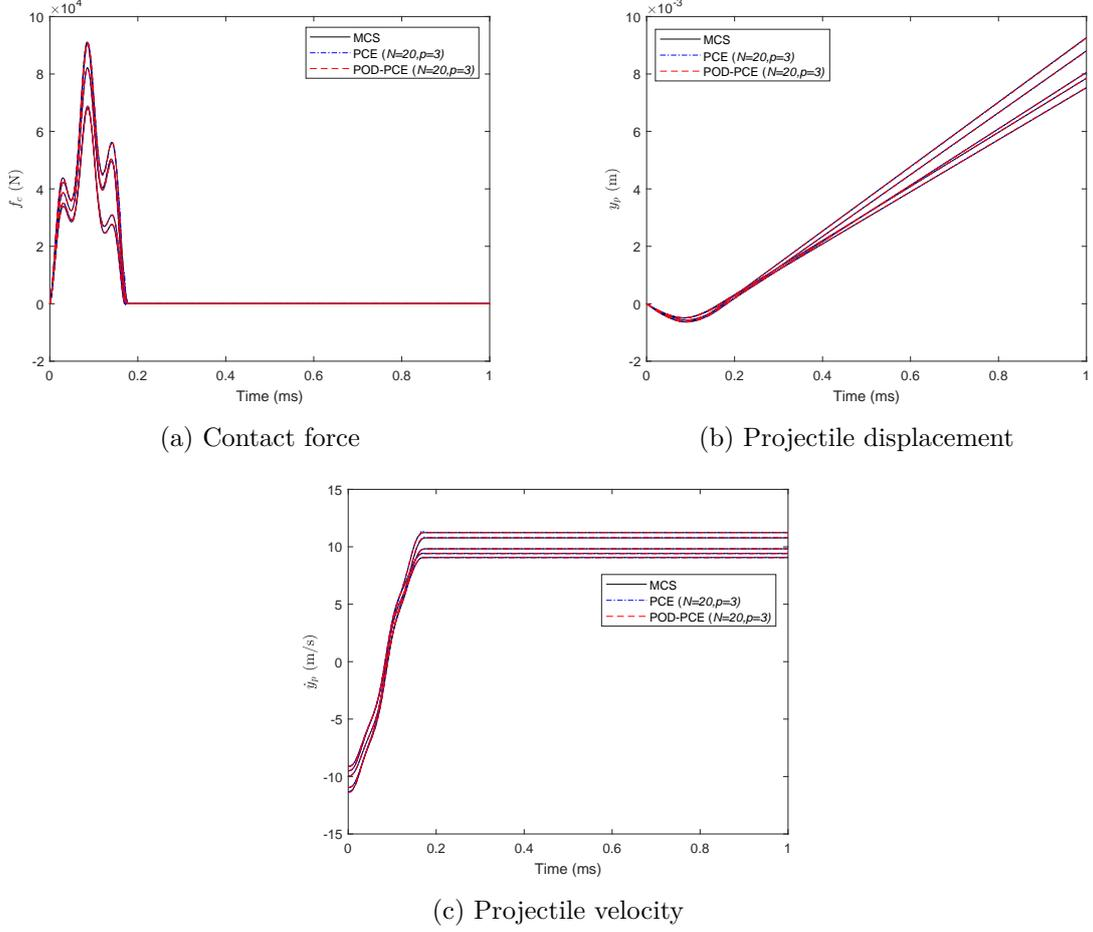
Figure 4.4: Comparison of responses for single impact oscillator at 5 samples:  $m_p \in \{342.71, 292.84, 365.62, 310.35, 373.82\}g$ ,  $k_c \in \{13.97, 13.87, 14.61, 14.23, 13.63\} \times 10^3 \text{MN m}^{-3/2}$ ,  $v_0 \in \{-11.32, 9.51, 9.96, 9.11, 10.95\} \text{m s}^{-1}$
