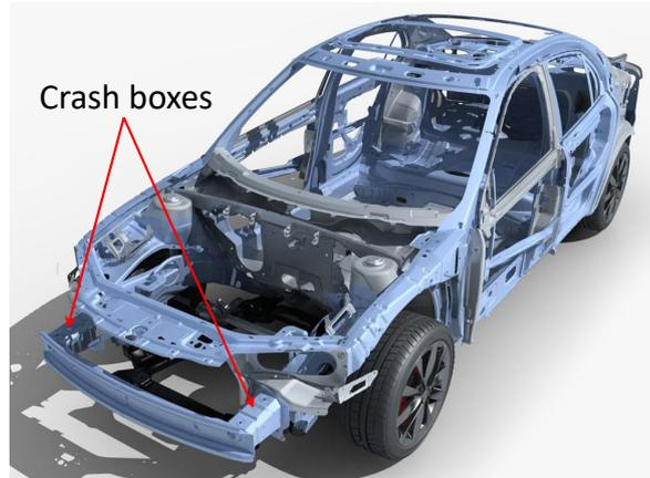
Figure 1.1: Frame structure of a car body ([www.cgtrader.com](http://www.cgtrader.com))
