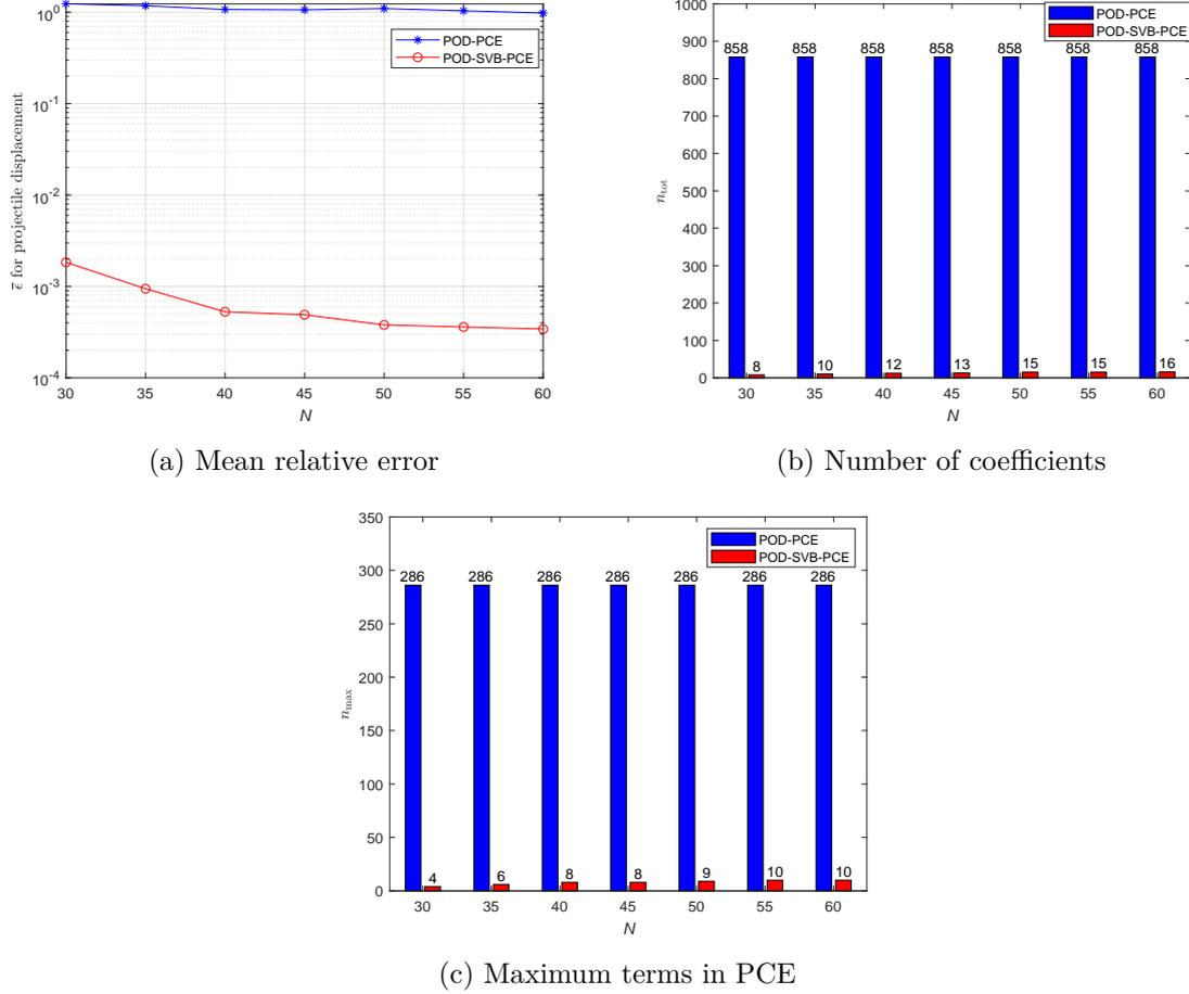
Figure 5.14: Evaluation of the mean relative error with the increase of sample point  $N$  for the predicted projectile displacement by the POD-PCE and the POD-SVB-PCE models with  $p = 10$
