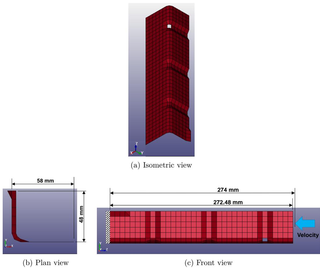
Figure 6.3: Geometrical views of FE model of the quarter crash box
