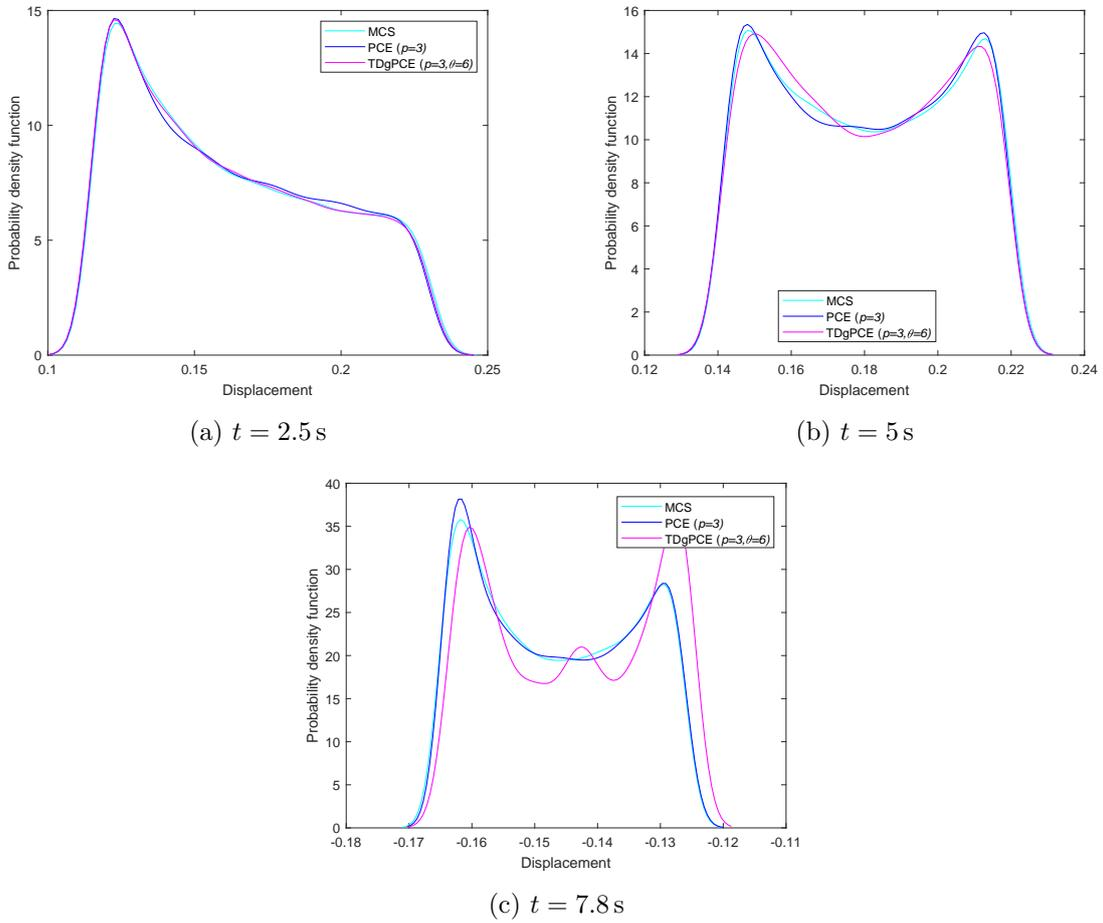
Figure A.3: PDF of displacement at different time instances for  $\bar{k} = 150 \text{ N m}^{-1}$
