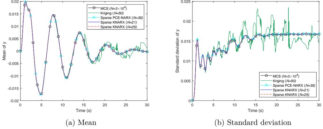
Figure 3.3: Statistical response characteristics of the Duffing oscillator
