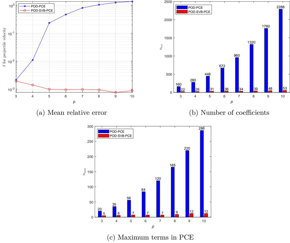
Figure 5.15: Evaluation of the mean relative error with the increase of polynomial degree  $p$  for the predicted projectile velocity by the POD-PCE and the POD-SVB-PCE models with  $N = 50$
