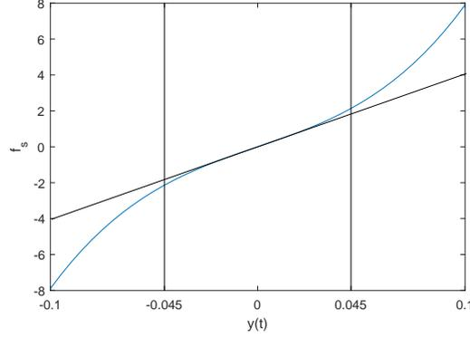
Figure 3.1: Displacement versus restoring force plot (blue curve) for the Duffing oscillator
