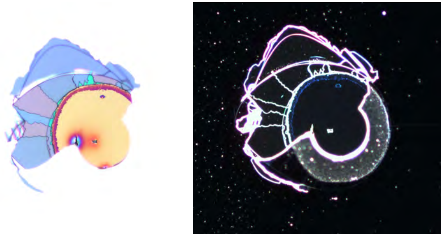
Figure 4.53: Center of the first supplied cylindrical mirror after lithography and laquer cap removal, observed with an optical microscope in white light (right) and in dark field (left).
