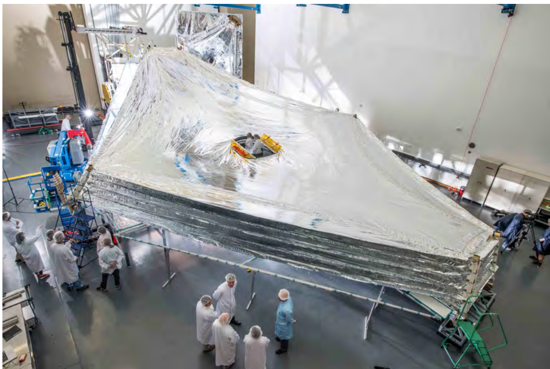
Figure 1.30: Sun shield of the JWST being tested at Northrop Grumman Corporation’s Space Park facility. Its size is that of a tennis court: approximately 20 meters long per 15 meters large. Source: NASA.
