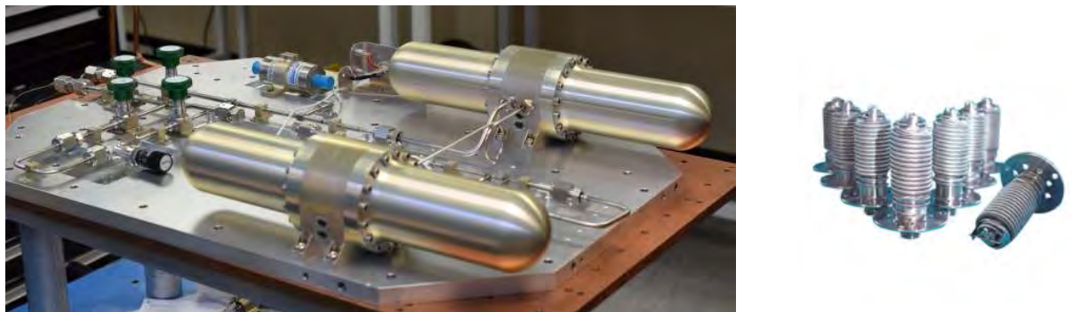
Figure 1.18: Left: J-T cryocooler cooling down a temperature of 2 K. Source: RAL. Right: J-T micro-coolers manufactured by Air Liquide Advanced Technologies [20].
