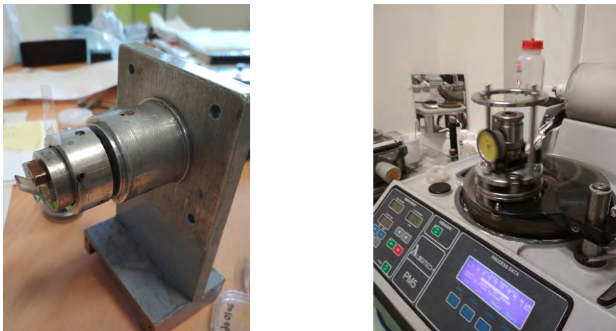
Figure 4.58: Left: Photograph of the crystal attached at the left to a goniometer head in order to precisely orient its c-axis on the Laue diffractometer. Right: Photograph of the crystal polishing step. The polishing head is rotating on a fabric plate with diamond powder.
