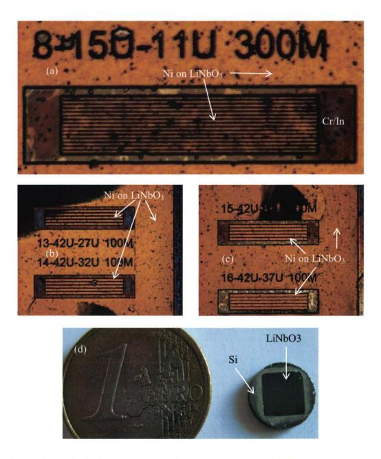
Figure 4.3.3: Optical microscope images of the realized LiNbO<sub>3</sub> arrays (with a thickness of 16  $\mu$ m) etched by ICP: (a) pitch = 15  $\mu$ m, kerf = 4  $\mu$ m for pattern 8 (b) pitch = 42  $\mu$ m, kerf = 15  $\mu$ m for pattern 13 and kerf = 15  $\mu$ m for pattern 14 (c) pitch = 42  $\mu$ m, kerf = 7  $\mu$ m for pattern 15 and kerf = 5  $\mu$ m for pattern 16 (d) fabricated sample compared with a piece of one euro.
