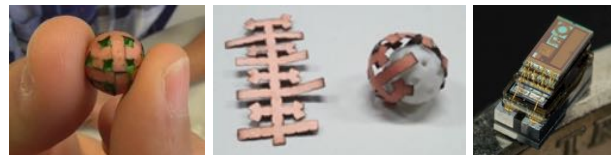
Figure 9.5: Current prototype of one of Julien Bourgeois 's \varnothing 11\text{mm} micro-robots (left), that can connect and roll around each other, thanks to their wrapped circuit (center) and embedded hardware (right), here shown on the edge of a coin. Future joint work will explore, among others, smaller ( \varnothing 3\text{mm} ) micro-robots, equipped with further sensors for interaction.
