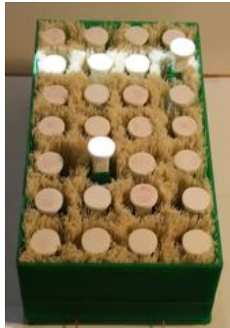
(b) Low-resolution emergeable prototype, with projection to highlight a raised slider (top) and dial (bottom).
