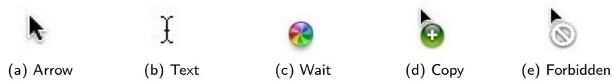
Figure 1.2: Five shapes given to the mouse cursor through software in order to provide feedforward to the user and, e.g., more accurate control with the thin text cursor.
