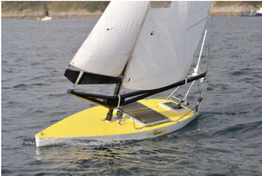
Figure 8.7: The VAIMOS drone: a basis for an un-manned surface vehicle aiming to autonomously deploy and recover Argo floats.
