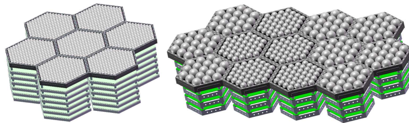
Figure 11. CAD drawing of the proposed POLARBEAR-2 focal plane (left) and LiteBIRD focal plane (right). POLARBEAR-2 focal plane mounts seven hexagonal wafers with lumped diplexer with total of 7588 bolometers. LiteBIRD focal plane uses two types of detectors. There will be eight low frequency wafers with larger lenses and five high frequency wafers near the center of the focal plane. LiteBIRD focal plane will have 2022 bolometers total.
