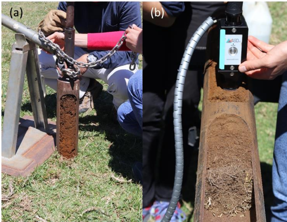
FIGURE 3.2 : IN SITU EXTRACTION OF SOIL CORE (A) AND IN SITU MEASUREMENT OF VNIR SPECTRA (B)
