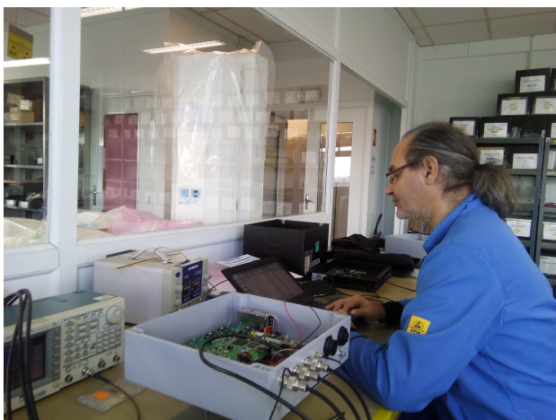
Figure 6.12: Left: David Martin testing one of the 35 Front-End unit produced at STAE in November 2017. Right: average signal levels measured at the outputs of the unit b07 for a sine wave of fixed amplitude and variable frequency. A relative variation smaller than 10% was found in the range 35-95 MHz for a majority of units.
