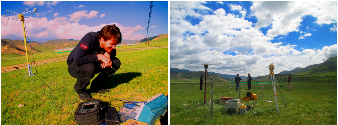
Figure 5.19: Left: Pierre Chauveau, intern on TREND in 2013, checking the quality of the sinus wave fed into the emitting antenna placed behind him during a PDTC measurement. Right: setup used for the TREND absolute calibration: the same bi-conical antenna as for PDTC is flown by a balloon filled with Helium gas and fed by a sine wave. The emitter position is steered with four ropes handled at ground and measured with a theodolite visible in the foreground. The TREND50 antenna being calibrated can be seen in the left of the picture.
