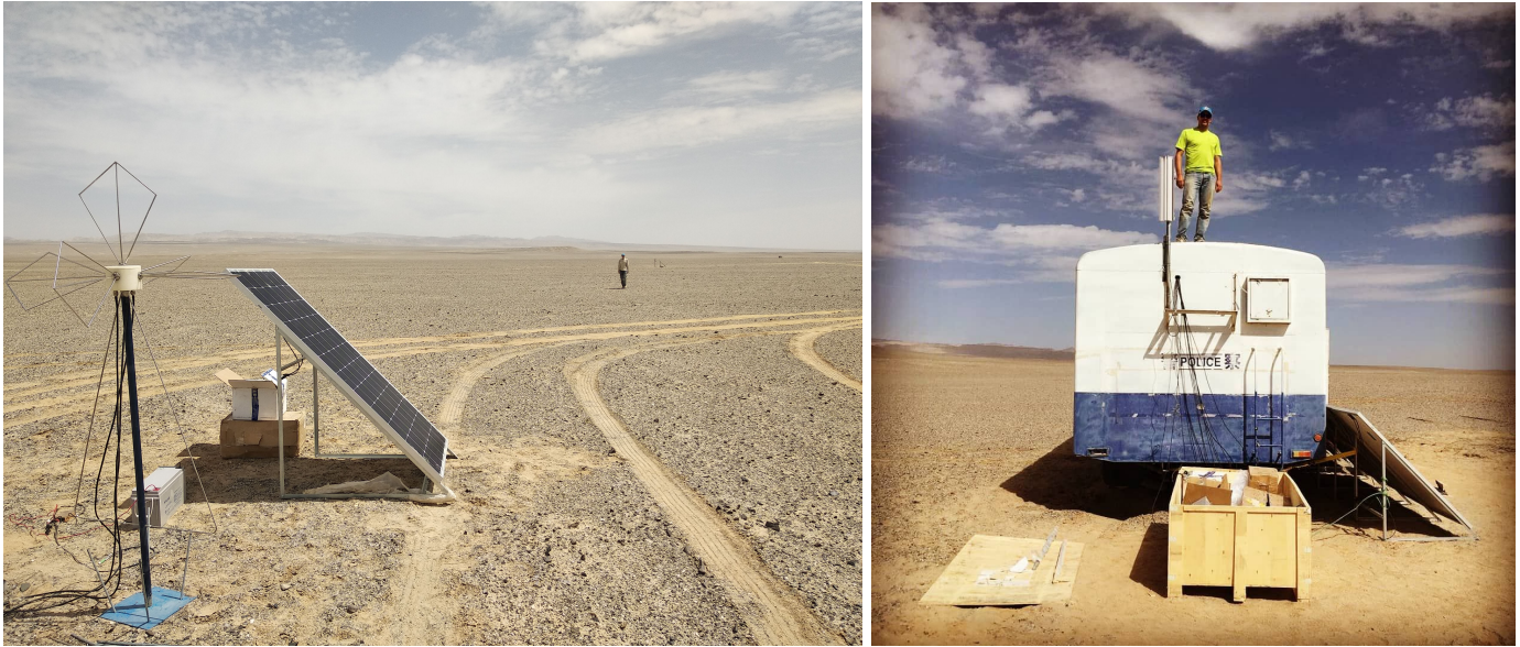
Figure 7.8: Left: Charles Timmermans walking towards one of the stations deployed for the long term measurement. A second unit can be seen behind him, and the black dot further right is the FTP. The noisy charge controller is the small metallic box lying on the ground, connected to the battery and the solar panel. Right: setting up the Rocket antenna atop the Field Termination Point.
