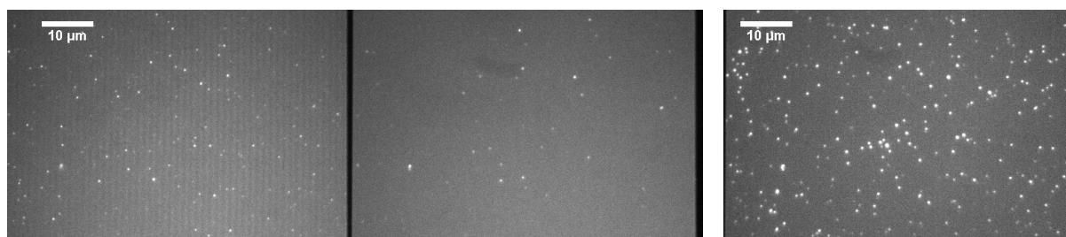
(a) Dual View image at excitation 488 nm: Donor channel on the left, FRET channel on the right. (b) Image at excitation 638 nm: Acceptor channel.
