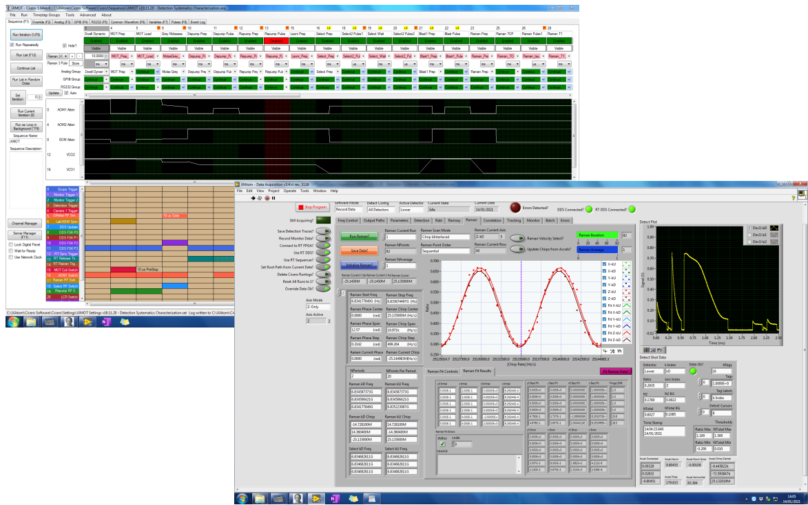
Figure 3.16: Screenshot of the two softwares operating the experiment. Cicero is used to control the sequence and LabVIEW to acquire signals and communicate via serial ports.
