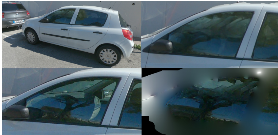
Figure 4.12 – Top left: novel view rendering with our method. Top right: crop of the view; rendering artifacts are visible. Lower left: closest input view; there is a strong discontinuity on a bright background with some reflections present. Lower right: reflection layer min-composite in this case.
