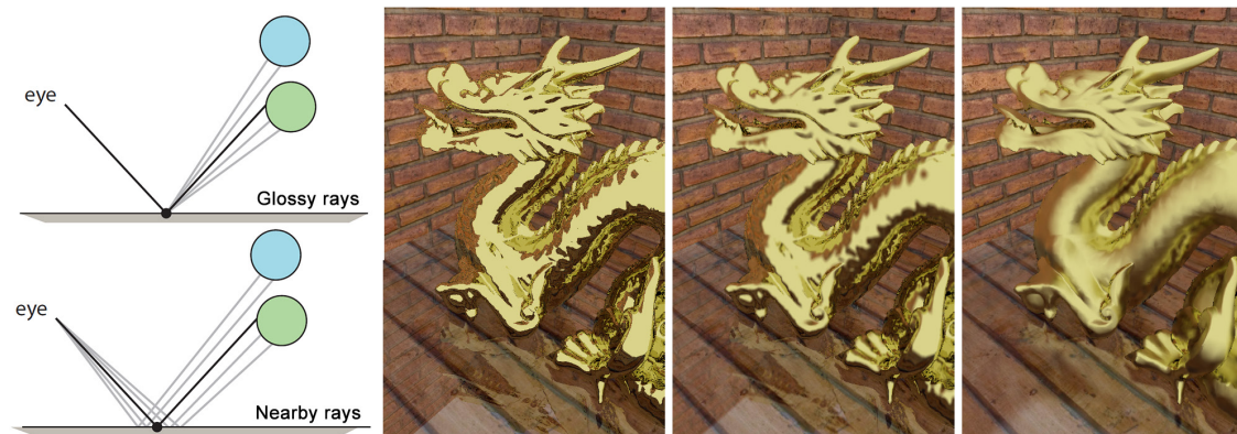
Figure 2.29 – Image-space gathering [RS09] approximates glossy reflections by using nearby perfect mirror rays (bottom left). Generated images using different roughness levels (right).
