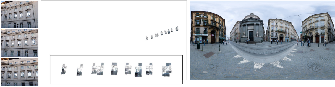
Figure 3.16 – Input images (left) and the resulting environment map after reprojection of the extracted reflections (center, zoom as inset). We use this incomplete environment map to select a similar one from a light probe dataset (right).
