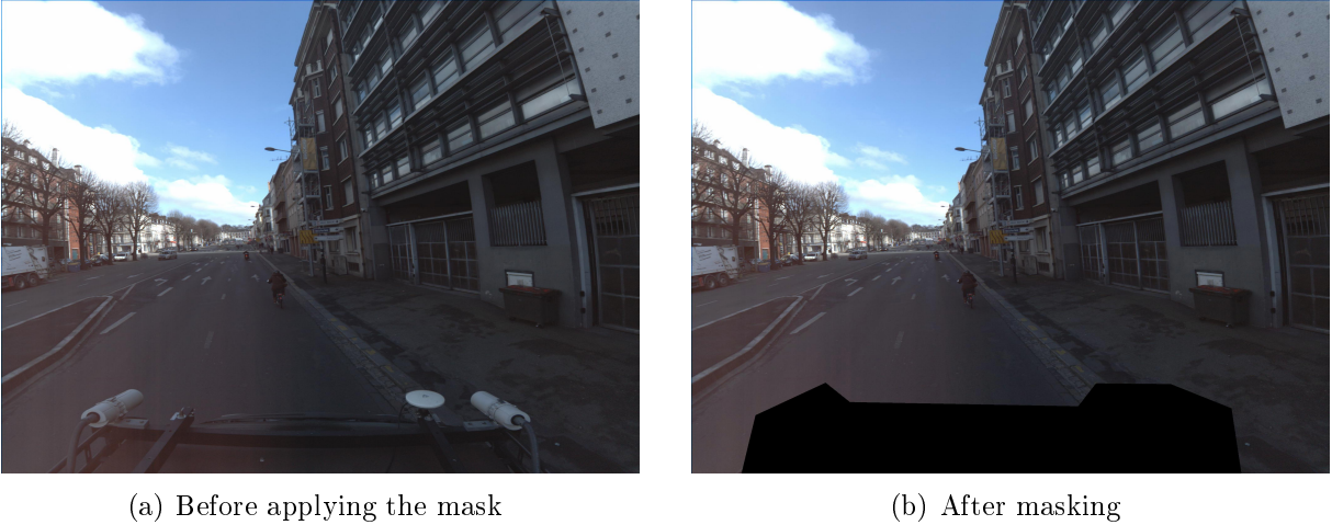
Figure 3.11: A mask is automatically applied on the collected images to avoid using the visible part as a texture for the final model
