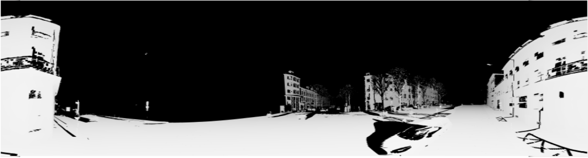
Figure 2.14: The reconstructed depth map at different maximum ranges. Distant buildings appears at a maximum range of 100 meters
