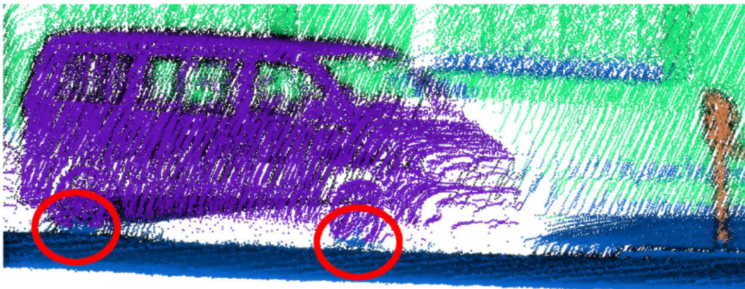
Figure 2.5: Illustration of the annotation inaccuracies from [48]: Wheels of the vehicle are confused with the ground
