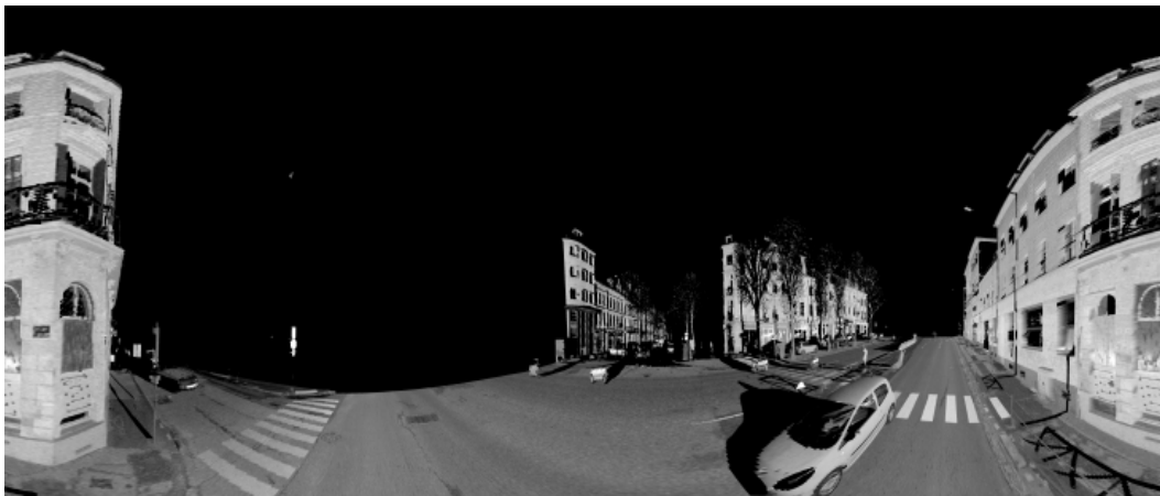
Figure 2.15: Illustration of the obtained LiDAR intensity map
