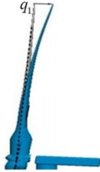
Figure 4.1 – Blade#1 flap-wise bending deflection.
