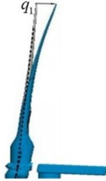
Figure 4.1 – Blade#1 flap-wise bending deflection.
