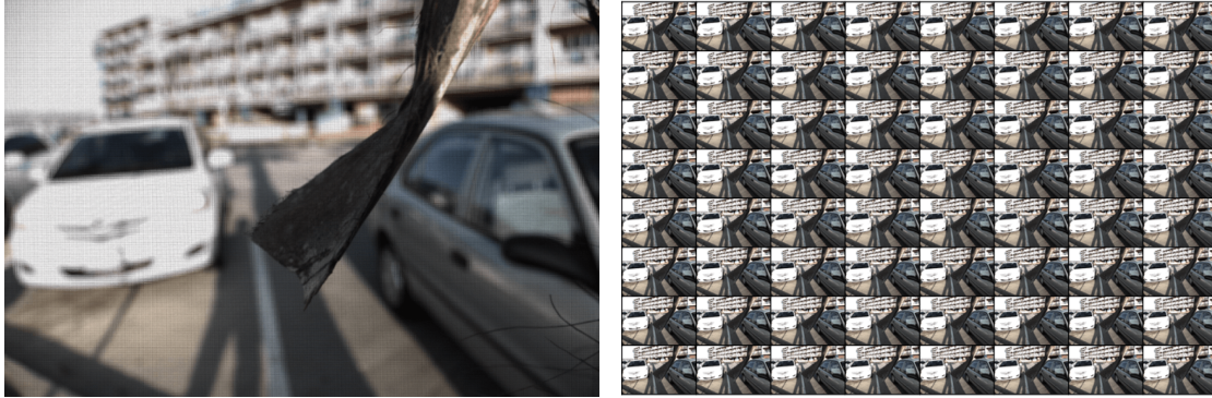
(a) Lumigraph obtained with a plenoptic camera (b) 8 \times 8 sub-aperture views obtained by re-organizing pixels of a lumigraph
