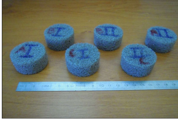
Figure III.5: Samples used for the characterization of the resistivity and acoustic properties.
