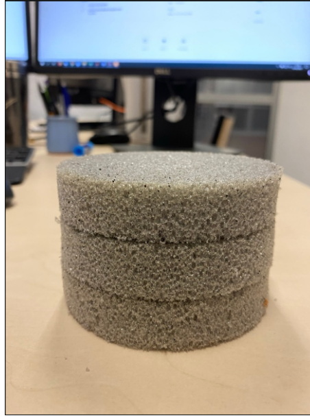
Figure III.3: Stack of samples used for the measurement of the open porosity and mass density.
