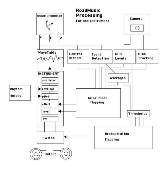
Figure 0-2: Schema of RoadMusic analysis and audio processing
