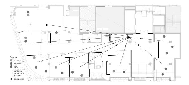
Figure 7-7: Stuart Jones, Sensor and speaker layout for Bop! 2005-2007.
