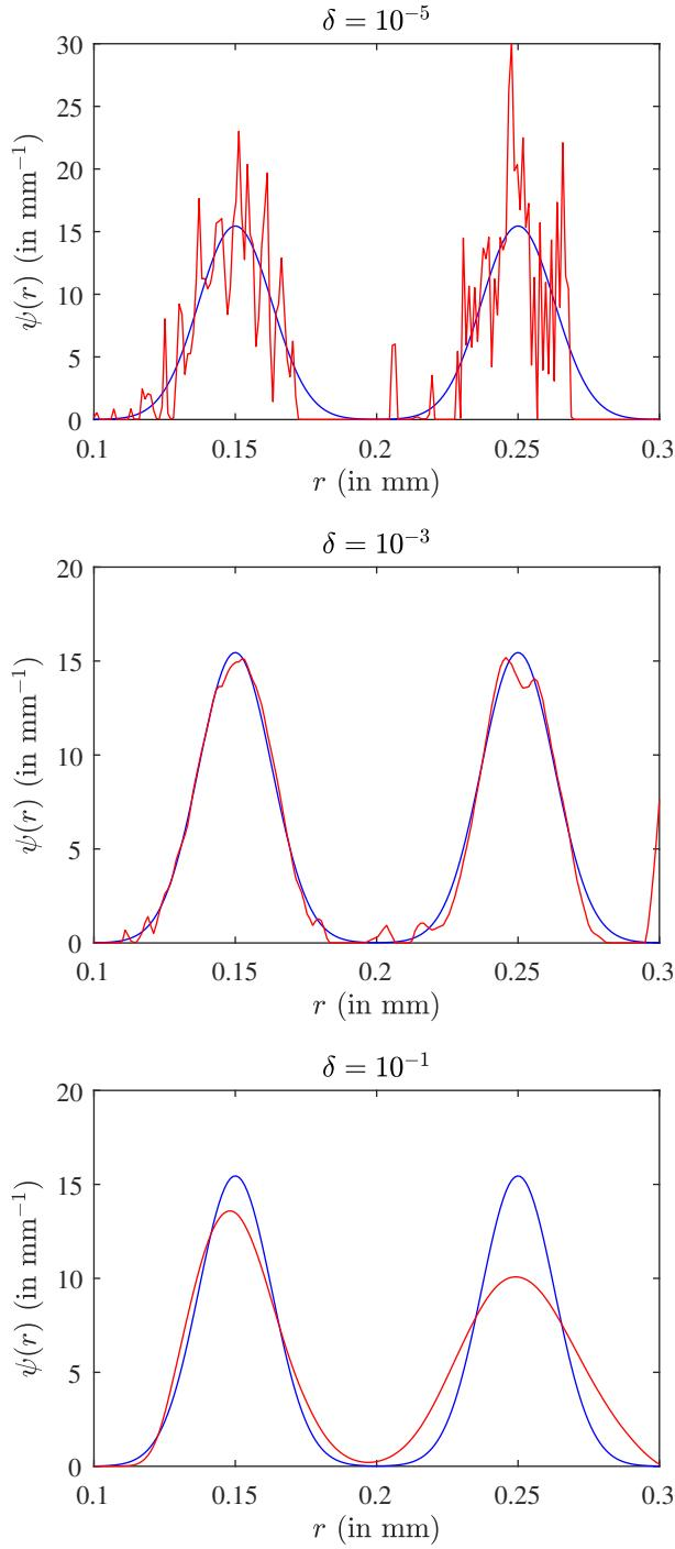
Figure 7.5 – Estimation of the PSD by the Tikhonov regularization method. In blue: the PSD given by (7.43). In red: the PSD estimated by the Tikhonov regularization method for  $\delta = 10^{-5}, 10^{-3}, 10^{-1}$ .
