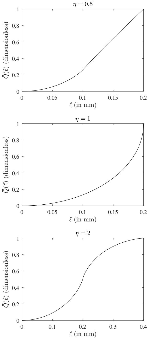
Figure 7.4 – Normalized CLD  $\bar{Q}$  associated to a Dirac distribution of spheroids at  $r = 1\text{mm}$  for  $\eta = 0.5, 1, 2$ .
