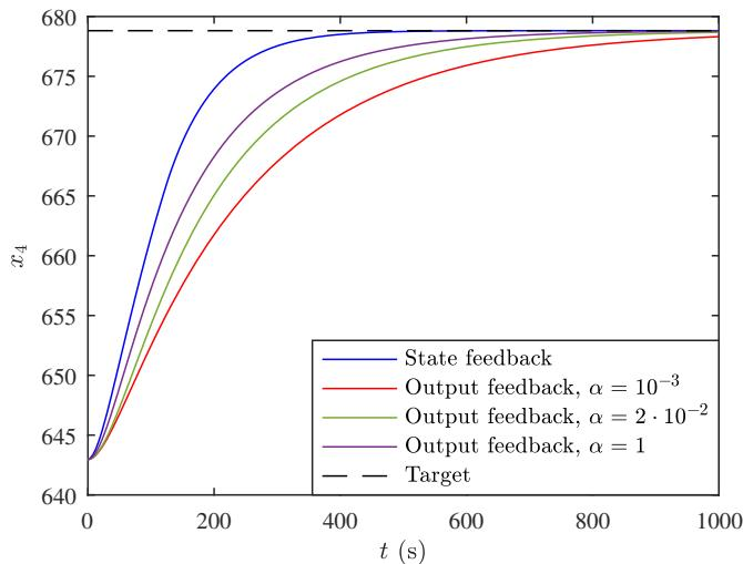
Figure 3.5 – Output enthalpy of the heat exchanger with the state feedback law  $\lambda$  and with the corresponding dynamic output feedback law based on the Luenberger observer for different values of  $\alpha$ .
