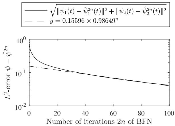
Figure 7.13 – Evolution of the absolute error between the actual PSDs  $\psi_1$  and  $\psi_2$  at time  $t = 1$  h and the estimations  $\hat{\psi}_1^{2n}$  and  $\hat{\psi}_2^{2n}$  obtained by (7.61)-(7.62) through iterations of the BFN algorithm.
