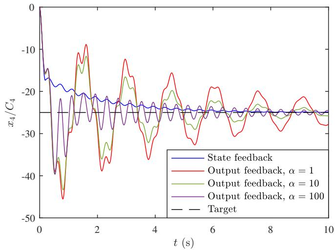
Figure 3.3 – Output voltage of the Ćuk converter with the state feedback law  $\lambda$  and with the corresponding dynamic output feedback law based on the Luenberger observer for different values of  $\alpha$ .
