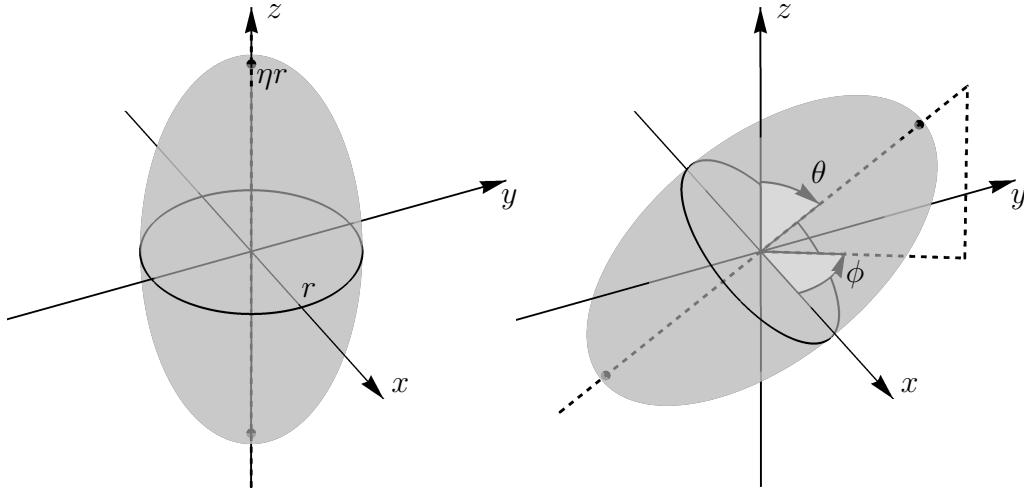
Figure 7.1 – *On the left:* elementary spheroid of parameter  $\eta$  and radius  $r$  (equation (7.15)). *On the right:* rotation of the elementary spheroid with angles  $\phi, \theta$  (equation (7.16))
