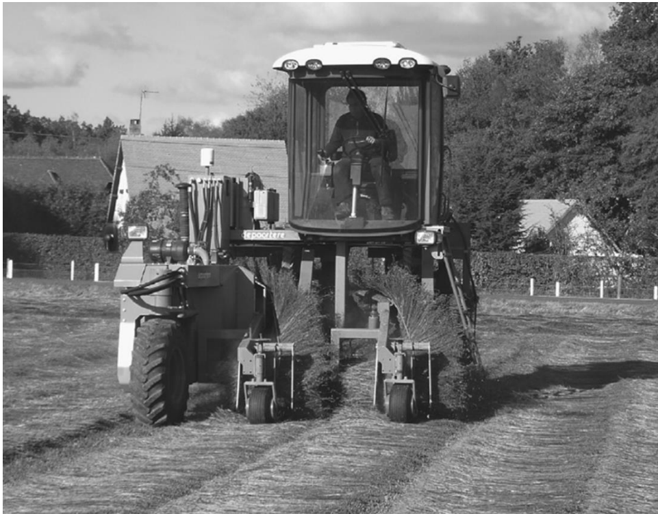
Fig. I - 11 Flax fibre dew-retting process (taken from [56])
