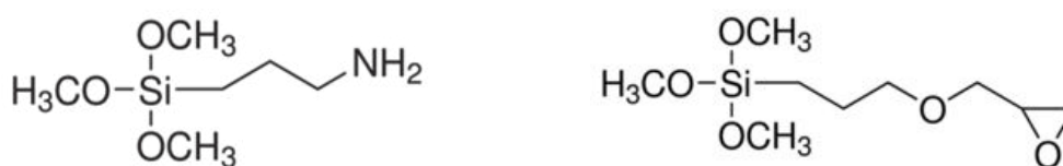
Fig. IV - 2 3-aminopropyltriethoxysilane (APS) and b) 3-glycidoxypropyltrimethoxysilane
