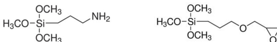
Fig. IV - 2 3-aminopropyltriethoxysilane (APS) and b) 3-glycidoxypropyltrimethoxysilane
