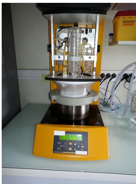
Fig. II - 2 Semi-automatic FIBRE THERM – GERHARDT® extractor used to determine the biochemical composition of flax fibres
