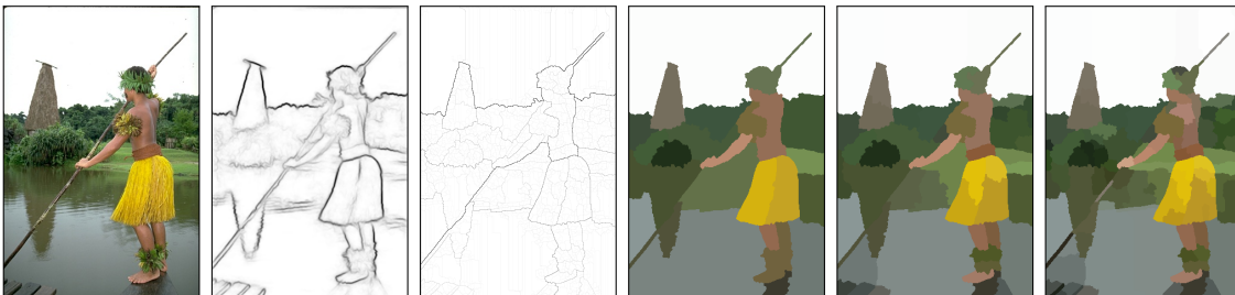
Figure 4.17: Example of image filtering with the proposed library Higura: image simplification with a watershed hierarchy. From left to right: original image, gradient, saliency map of the watershed hierarchy by area of the gradient, simplified image reconstructed from the hierarchy with respectively 25, 50, and 100 regions.
