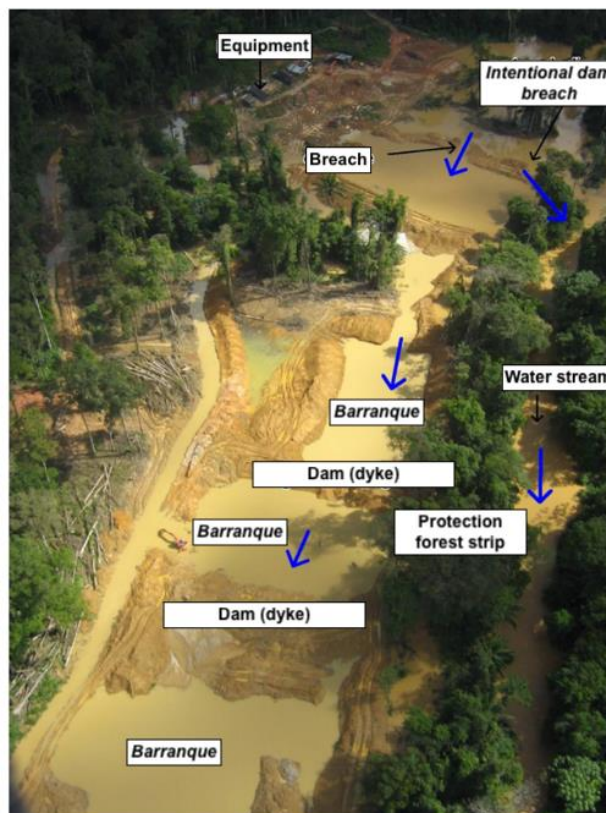
Figure 51 Example of a mining dam system in a secondary gold mining site (ASM-type) in FG (Barras, 2010)
