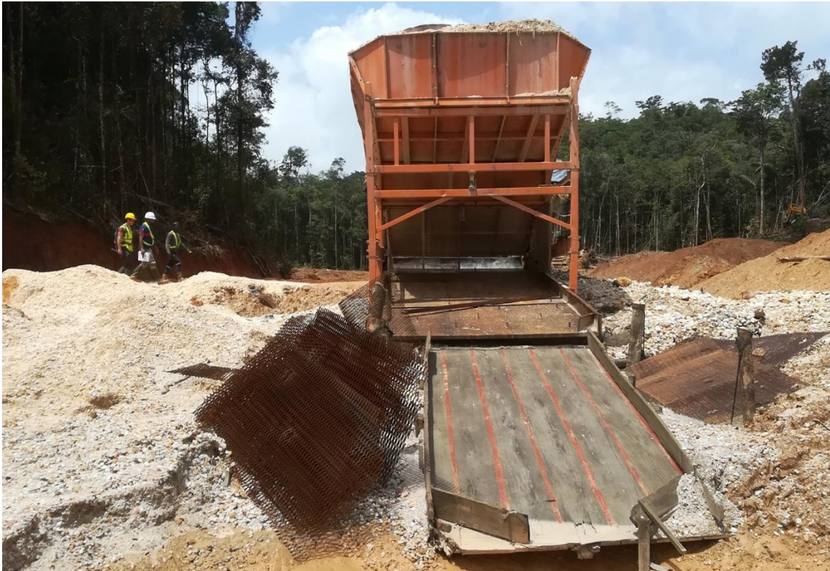
Figure 28 Settling-table for the first trapping of gold particles and the filtering of materials by grain-size. Location: western French Guiana
