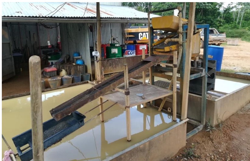
Figure 33 One of the several machines used for gold recovery of secondary gold mines by gravimetry. Location: eastern French Guiana
