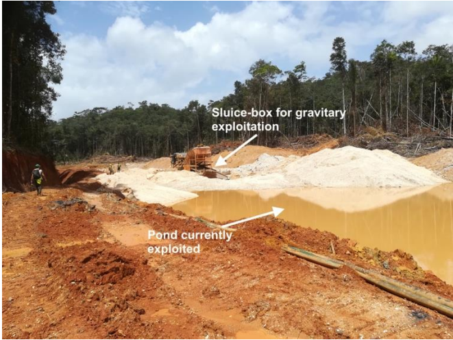
A mining dam system in a ASM project type. The pond currently exploited and the sluice-boxe used for gravitary exploitation
