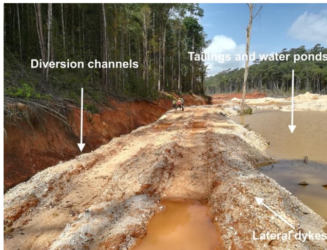
A mining dam system in a ASM project type. The ponds (barranques) are separated from the diversion channels by lateral dykes of few meters
