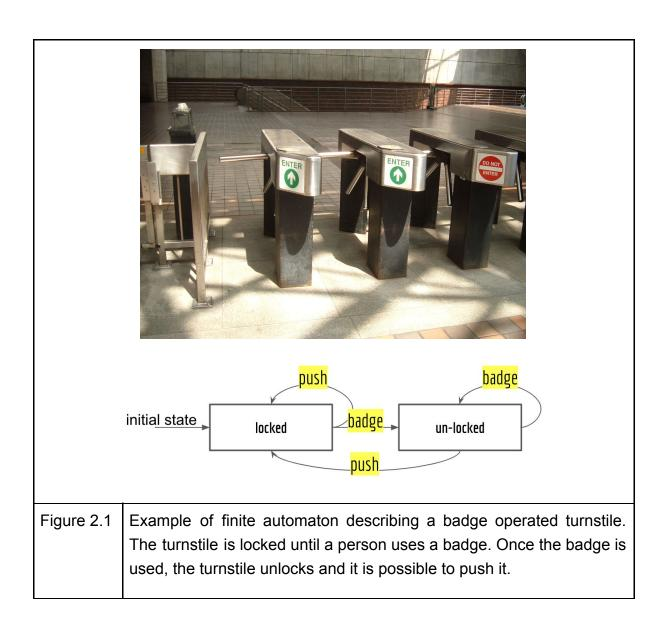
In Figure 2.1, we provide a basic example of automaton that describes the functioning of a turnstile. There are two **states** corresponding to the situations where the turnstile is locked, or unlocked. There are four **transitions**, represented by the arrows connecting the states or looping on one state. The **conditions**, which are the external inputs that determine the transition, are the user's actions: push or use the badge.
