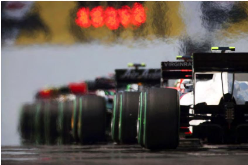
**Figure 1.4.** Heat haze: the heat produced by F1 engines is distorting the image captured by the camera. (Darren Heath ©)
