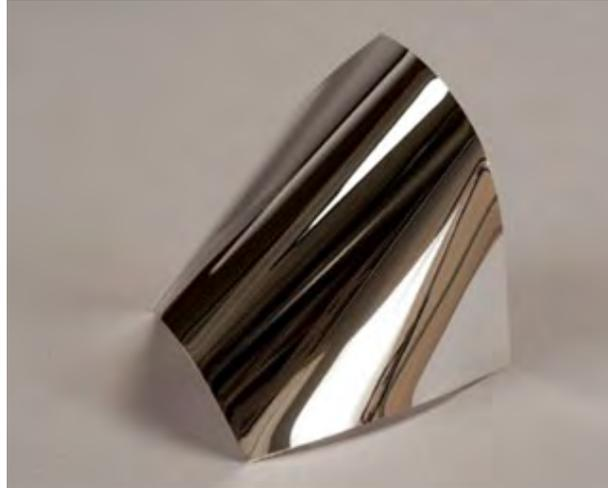
**Figure 4.35.** Film providing high specular reflection of visible light. (SirVisual ©)
