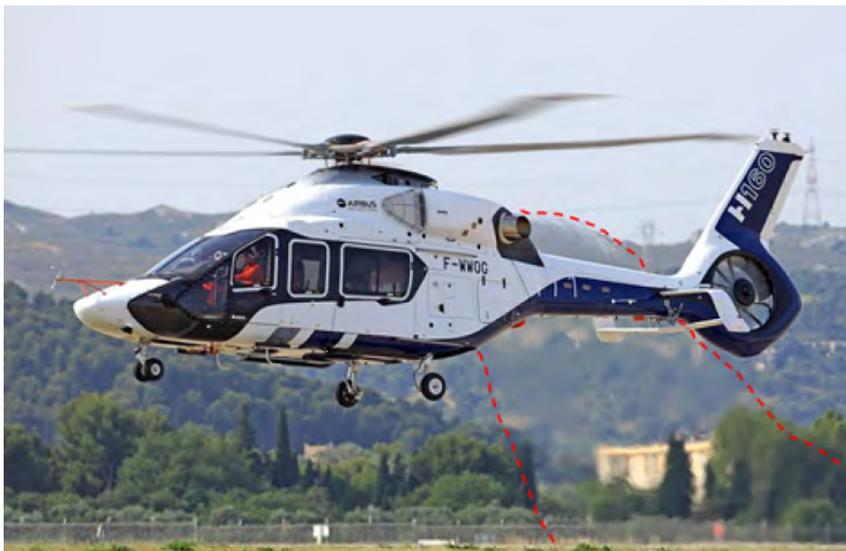
**Figure 4.1.** Engine exhaust gases visualization for an H160 helicopter hovering in ground effect. Between the red lines the heat produced by the engines warp the image captured by the camera. (Tatjana Obrazcova ©)
