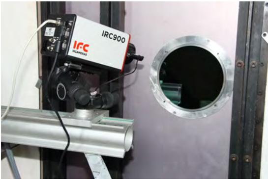
(b) Details of the infrared camera and the IR window.
