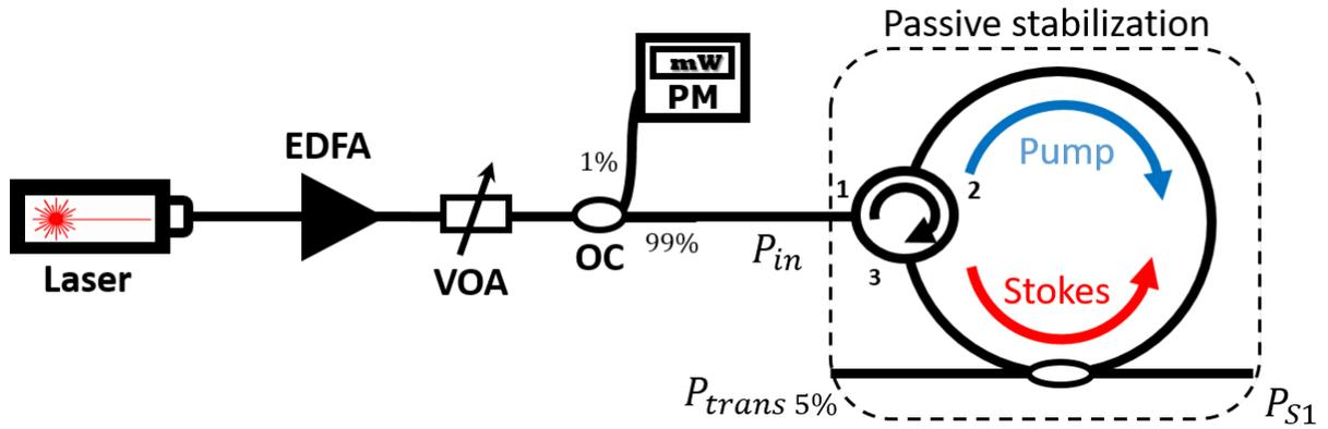
Figure 3.3: Experimental setup for non-resonant fiber ring cavity Brillouin laser characterization
