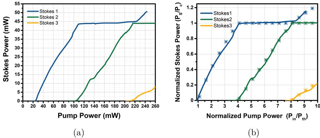
Figure 4.4: (a) Power characterization of  $MBL_{LQ}$  cavity (b) Normalized Power characterization of  $MBL_{LQ}$  cavity with its input power,  $P_c$ : clamping power,  $P_{th}$ : threshold power of S1
