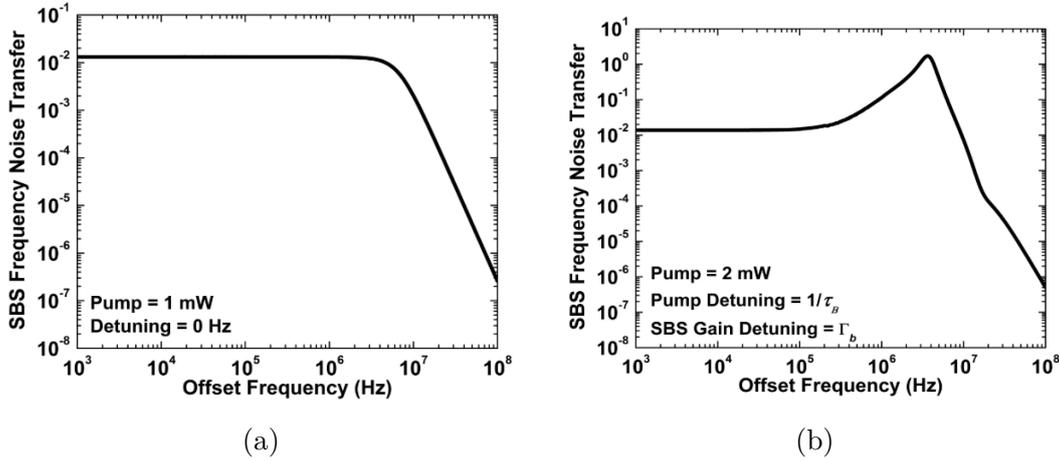
Figure 4.20: The pump frequency noise to Stokes frequency noise (a) zero detuning (b) with pump and SBS gain detuning [4].
