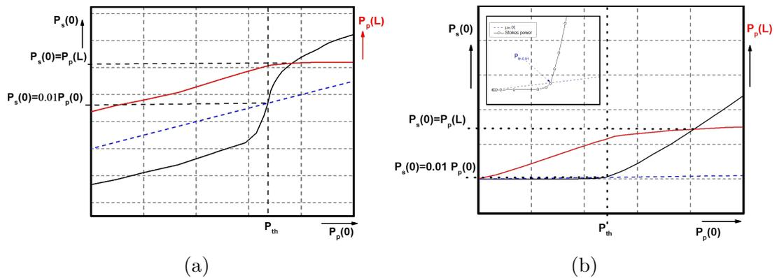
Figure 2.5: Definition of Brillouin threshold power using transmitted (red) and back-scattered Stokes (black) signals plotted as a function of the input power. 1 % of the input signal is plotted in blue color for references.  $P_p(0)$  : input pump power,  $P_s(0)$ : back-scattered Stokes,  $P_p(L)$ : transmitted power; (a) Logarithmic scale (b) Linear scale.
