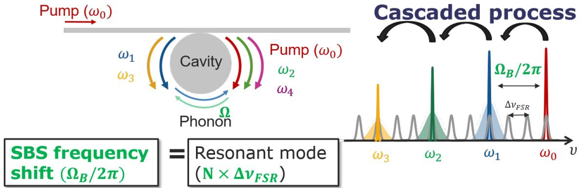
Figure 4.1: Illustration of cascade Brillouin laser. A pump laser of frequency  $\omega_0$  is injected into an optical resonator. When its wavelength matches the Brillouin condition ( $(\Omega_B/2\pi) = N \times \Delta\nu_{FSR}$ ), pump resonant mode at  $\omega_0$  is scattered at  $\omega_1$  by emitting a phonon at  $\Omega_B$ . When the pump power is sufficiently high, the Stokes wave at  $\omega_1$  acts as a pump for higher order Stokes lines.
