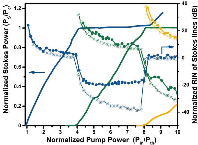
Figure 4.6: Left axis : Output Stokes power ( $P_s$ ) normalized to the circulating power ( $P_c$ ) versus input pump power ( $P_{in}$ ) normalized to the Stokes 1 lasing threshold ( $P_{th}$ ). Right axis: RIN of Stokes lines normalized to the input pump RIN. RIN amplitude is measured at 4 kHz from the carrier. Straight lines and full dots are experimental results. Stars are simulation results. Results are obtained with the "low-Q cavity" Brillouin laser,  $P_{th} = 26.5$  mW.
