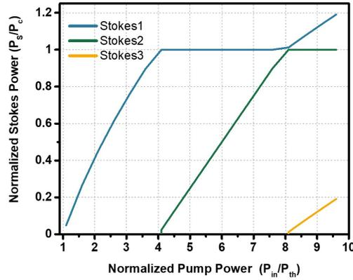
Figure 4.3: Steady-state laser powers for the Stokes components, obtained from the simulation.
