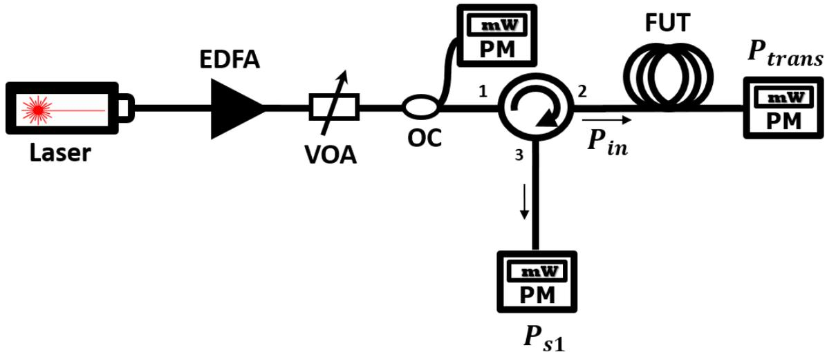
Figure 2.9: Experimental setup for SBS threshold measurement. EDFA: Erbium doped fiber amplifier, VOA: Variable optical attenuator, FUT: Fiber under test ( $L=26$  km), PM: Powermeter, OC: Optical coupler.
