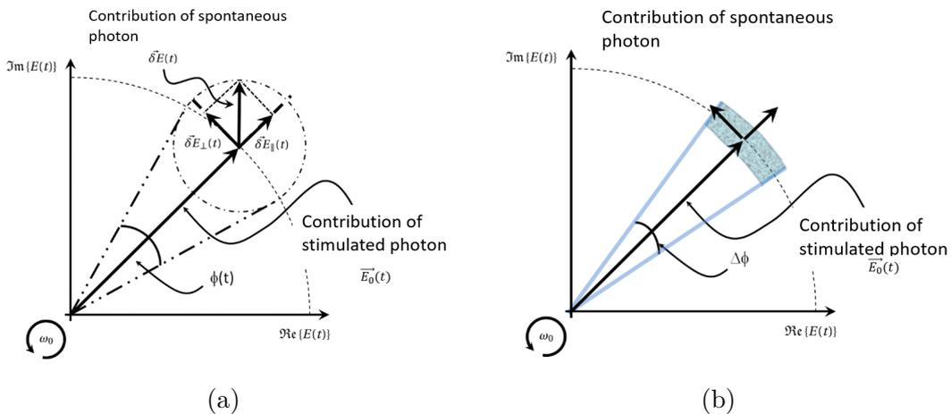
Figure A.1: (a) Schematic representation of spontaneous emission of laser field (b) Contribution of stimulated emission generated by optical amplification and filtered by an optical cavity.
