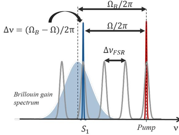
Figure 4.11: Schematics presentation of gain detuning of Brillouin cavity.
