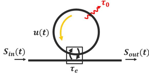
Figure 2.11: Schematic view of the resonator.  $S_{in}(t)$  : input field,  $S_{out}(t)$  : output field,  $u(t)$  : resonant field,  $\tau_0$  : intrinsic photon lifetime,  $\tau_e$  : coupling lifetime.
