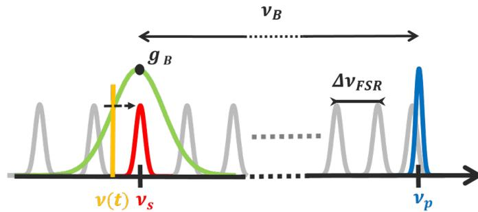
Figure 2.15: Spectral overview of the CRDM method: Pump laser line (blue), Brillouin gain curve (green), probed cavity mode (red) and probing laser line (yellow).  $\nu_B$  corresponds to the Brillouin shift, where  $\Delta\nu_{FSR}$  stands for the spectral spacing (Free Spectral Range) between cavity modes.
