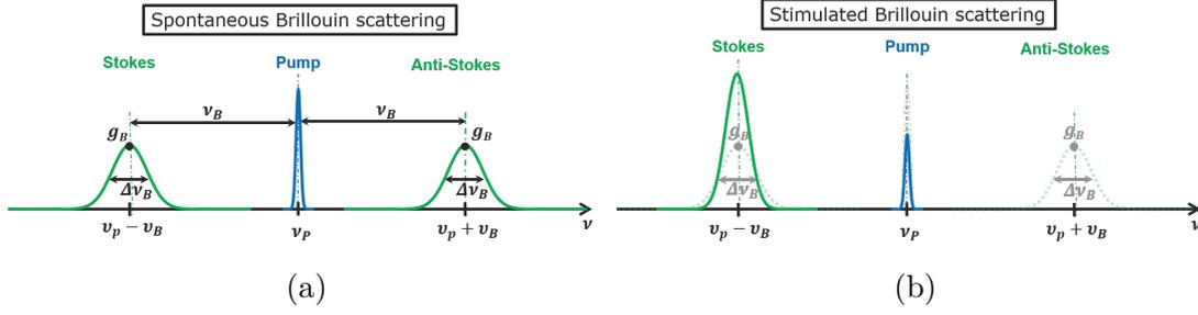
Figure 2.2: Stokes process in (a) the spontaneous regime. Amplitudes of Stokes and anti-Stokes are of same order. (b) Stimulated Brillouin scattering regime. Stokes amplitude will increase and its gain spectrum narrows.  $\nu_B$ : Brillouin shift,  $\nu_P$ : pump frequency,  $\Delta\nu_B$ : Brillouin gain bandwidth and  $g_B$ : Brillouin gain coefficient
