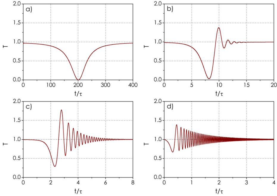
Figure 2.13: Transmission of a resonator for different scanning speeds. (a)  $\tilde{V}_S=0.0075 \tilde{V}_0$ , (b)  $\tilde{V}_S=0.3 \tilde{V}_0$ , (c)  $\tilde{V}_S=3 \tilde{V}_0$ , (d)  $\tilde{V}_S=30 \tilde{V}_0$  with a  $\tilde{V}_0 = 2/(\pi\tau^2)$  [1].
