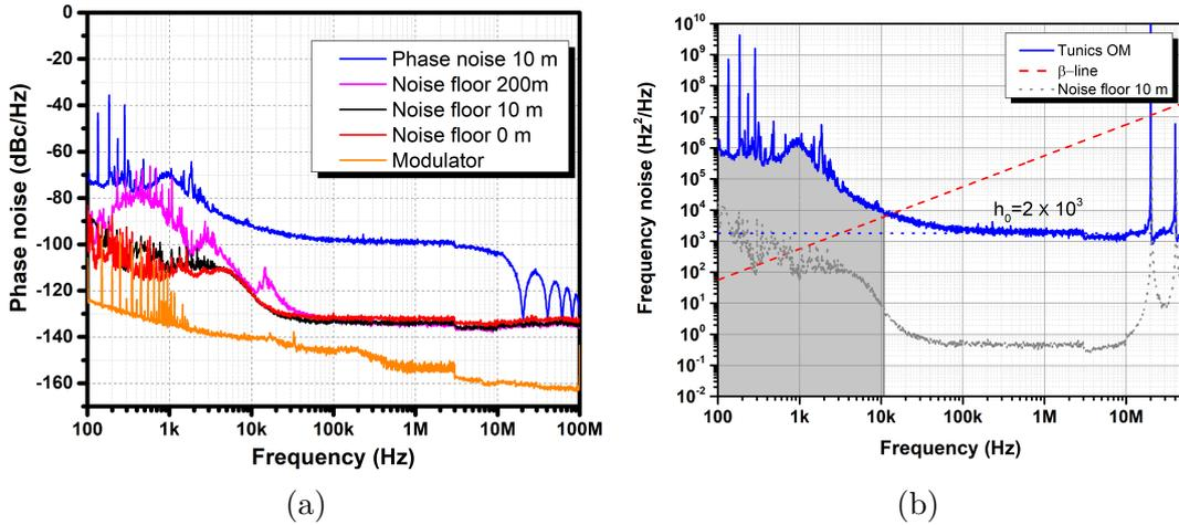
Figure 1.8: (a) Phase noises of the laser and noise floors of the bench for different fiber lengths. (b) Frequency noise measurement of the Tunics OM laser and its linewidth estimation using  $\beta$  – line approximation.
