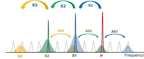
Figure 4.16: Schematic of anti-Stokes generations in cascaded Brillouin laser; dotted line : resonance of the cavity; shaded spectrum are Brillouin gain profiles for Stokes and anti-Stokes: S1 (blue), S2 (green), S3 (yellow); sharp peaks are Stokes stimulated laser lines and pump (green for S2, blue for S1, red for the pump).
