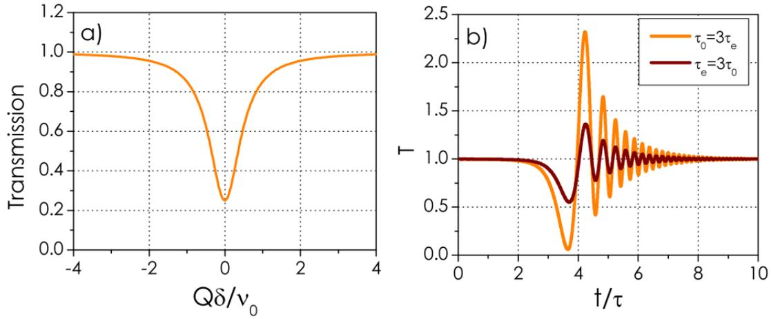
Figure 2.14: (a) Transmission in the stationary regime as a function of the normalized detuning in the case of  $\tau_0 = 3\tau_e$  and  $\tau_e = 3\tau_0$ . The two curves are exactly superimposed. (b) Transmission as a function of time in the same two cases with  $V_s = 2.25V_0$ . Note that the two responses are easily distinguishable [1].
