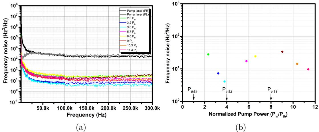
Figure 4.18: Cascaded Brillouin laser frequency noise dynamics (a) S1 frequency noise at different pump powers in linear scale (b) S1 white noise at a fixed frequency of 200 kHz as a function of normalized pump power.
