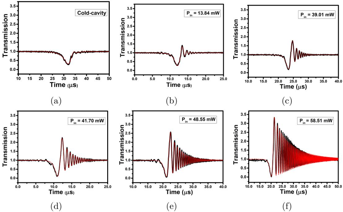
Figure 2.17: Fast scanning profiles recorded from the Brillouin cavity at different pumping power ( $P_{in}$ ) with a scanning speed of  $2.8 \text{ MHz}/\mu\text{s}$ : The intrinsic photon lifetime ( $\tau_0$ ), transmission and Brillouin gain coefficients are deduced from the analytical fits (red) of experimental curve (black). (a) cold cavity, (b) under coupling, (c) near to critical coupling, (d) over coupling, (e) near to transparency, (f) amplification.
