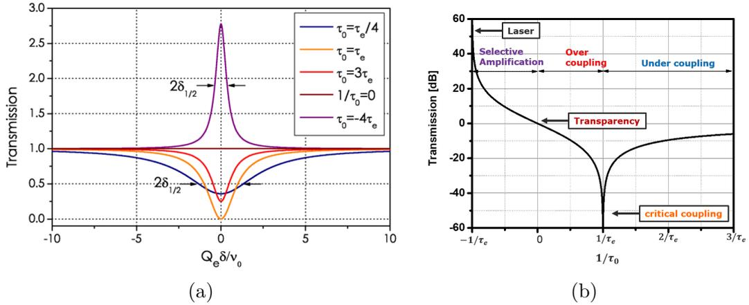
Figure 2.12: (a) Transmission spectrum in steady state for different relative values of  $\tau_0$  and  $\tau_e$  [1]. (b) Transmission at resonance  $T(\delta=0)$  in decibels as a function of  $1/\tau_0$  for the different coupling regimes.
