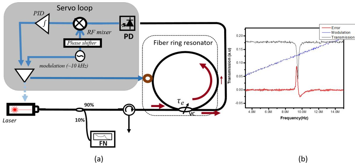
Figure 1.10: (a) General scheme of top-of-fringe frequency stabilization. (b) Oscilloscope traces for transmission laser signal, modulation and top of fringe error signals. PD: photodetector, PID: Proportional–integral–derivative controller, VC: Variable coupler, FN: Frequency noise measurement bench.
