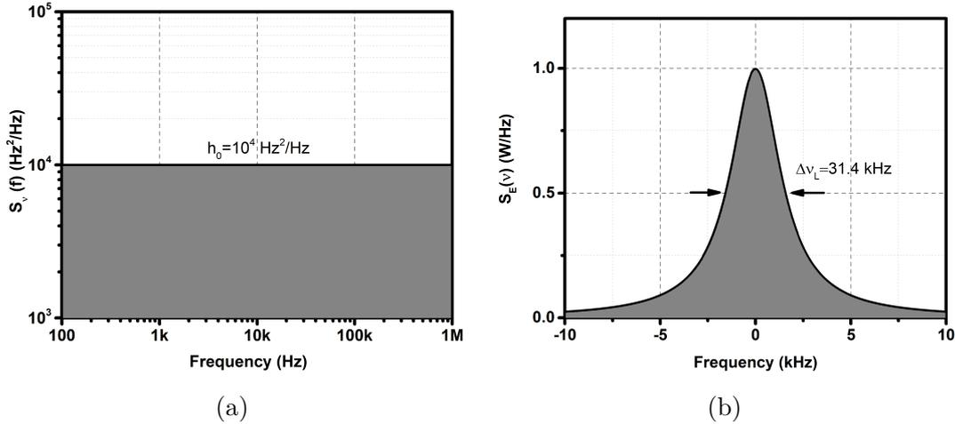
Figure 1.3: Illustration of corresponding frequency noise and optical spectrum. (a) Frequency noise  $S_\nu(f) = h_0 = 10^4 \text{ Hz}^2/\text{Hz}$ . (b) Optical spectral of the laser corresponds to the white frequency noise and the intrinsic linewidth  $\Delta\nu_L = 31.4 \text{ kHz}$
